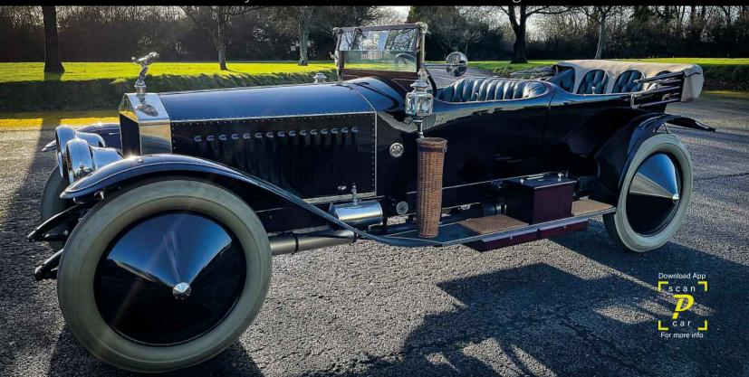
A fine and rare sporting Edwardian Ghost. Ordered as an L&E "colonial" specification chassis with Torpedo coachwork by Connaught. The colonial specification included 4 speed transmission, a more powerful high compression engine with lightweight pistons and a larger carburettor, a long range fuel tank, larger radiator and more. A perfect international touring car. Restored to the very highest standard.
