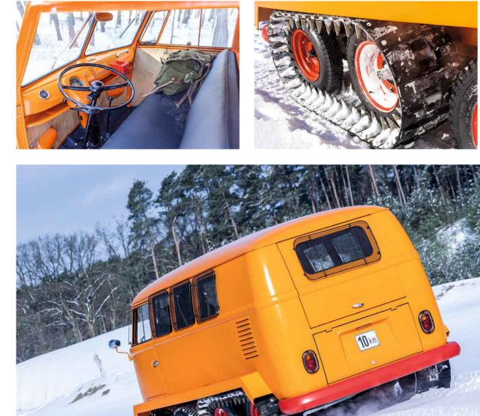
Clockwise, from top left Half-Track is limited to 35km/h on the road; front cockpit is standard Bulli; traction on snow is provided by specially made wheel-driven tracks; there's no stopping it.
