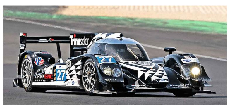
2012 ex-Dempsey Racing Lola B12/80 LMP2 Carbon fiber monocoque with Judd 3.6 liter V8 engine. Fully rebuilt in 2019 incl.-engine and gearbox. P.O.A
