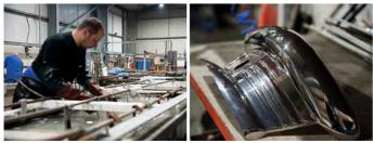
Most chrome-platers have done away with the dull nickel stage these days, but 'we do it the way it's always been done,' says Hayward, who explains that dull nickel's value is its excellent corrosion resistance. If S&T's checking and rechecking process is impressive, the attention to detail and sheer polishing work is stupefying as items go back and forth in the process until they are perfect and you can see your coffee-stained teeth in it.
