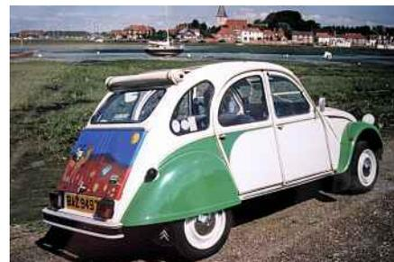
The brilliant, self-levelling suspension was described by an American writer as a 'tusk, lever, cable, push, pull cannister o'springs', a perfect description. Also, when fully laden, the wheelbase increases by two inches!
