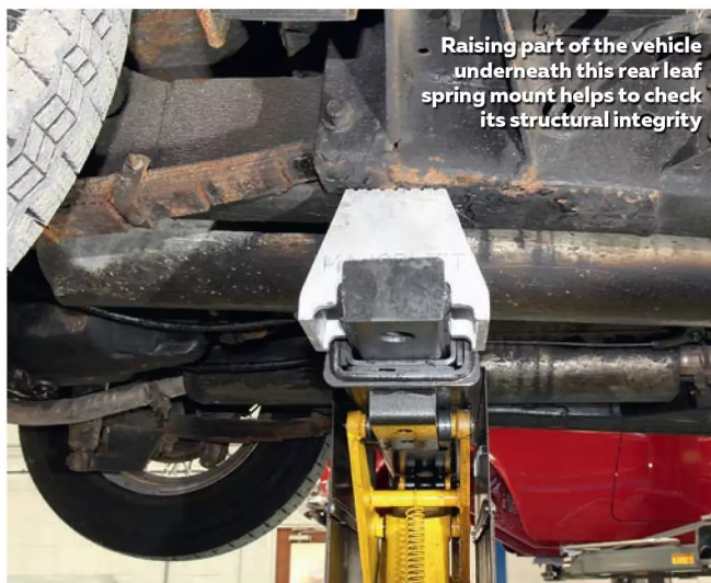
Chassis outriggers can be inspected from underneath to ensure they're in good order
