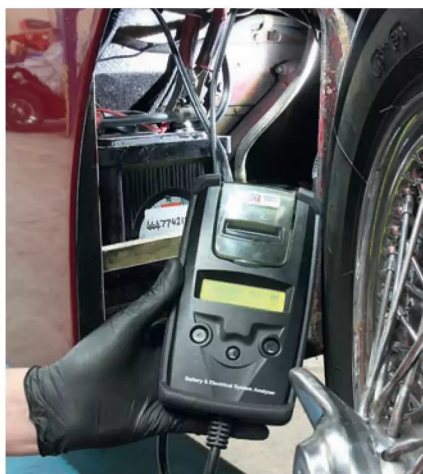
The original-spec six-volt batteries sit inside the front wings
