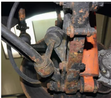
Front suspension includes telescopic dampers and an anti-roll bar, where the drop-link bushes can become worn and cause a knocking sound
