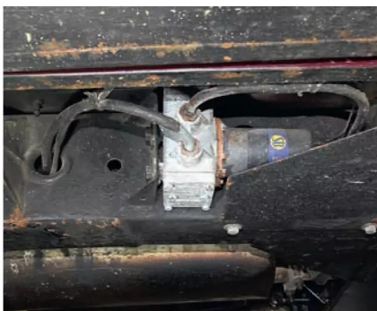
The electric fuel pump mounted underneath the XK150 should be inspected for leaks and corrosion
