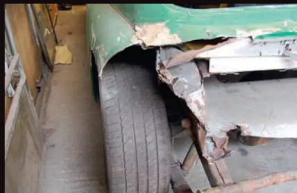
Cutting the rear wings away revealed the poor condition beneath the surface
