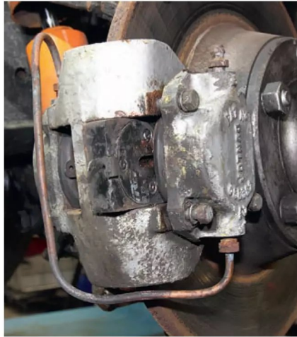
The braking system uses Dunlop twin-piston calipers all round; pads can become stuck, but partially removing the piston can help
