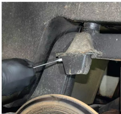
Look for a bump stop at every corner of the car; they protect the chassis when the suspension is fully compressed
