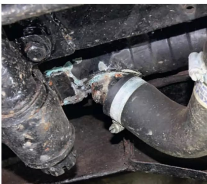
Potential buyers should inspect all coolant hoses for leaks and residue
