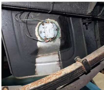
Petrol may have leaked past this sender unit on the side of the tank
