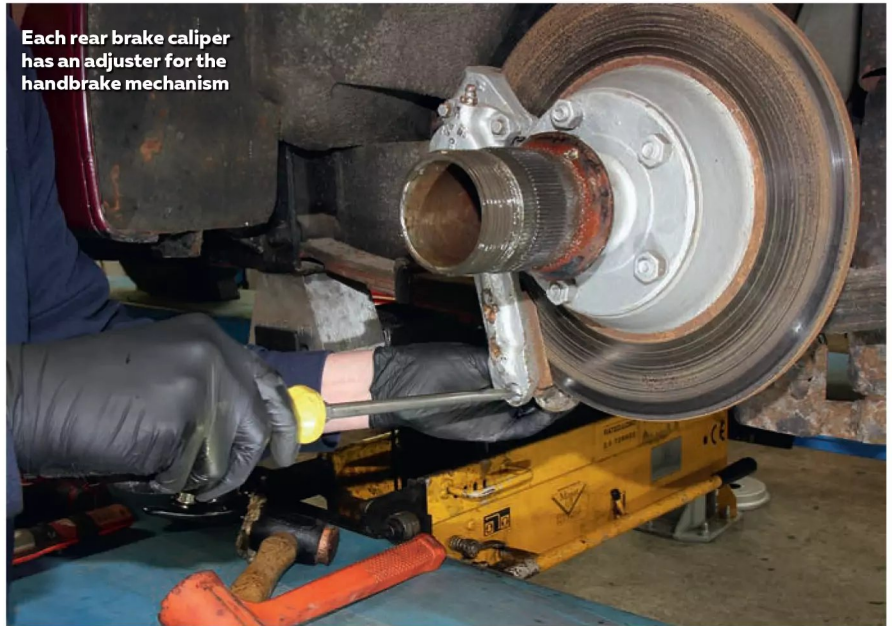
The braking system uses Dunlop twin-piston calipers all round; pads can become stuck, but partially removing the piston can help
