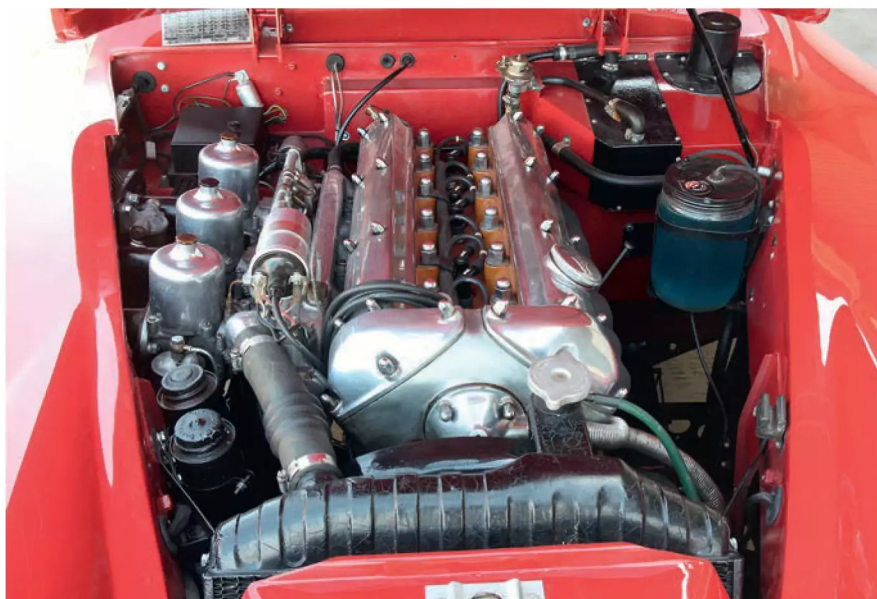
The 265bhp, 3.8-litre engine in the XK150 S is the ultimate performance motor for this model
