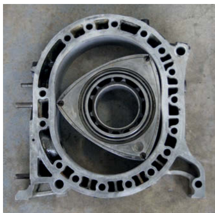
The rotor spins in this housing, hence rotor tip wear is an issue.
