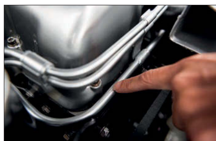
Engine recently rebuilt and engine bay overhauled. Parts supply was a big issue. This coolant pipe was made from scratch.
