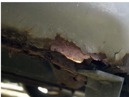
Sill rot is a major RX-8 issue.
