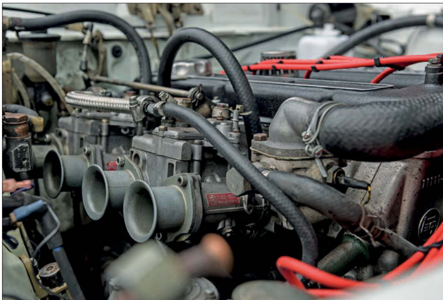
Twin carbs have very little filtering. Suspension (Right) uses Megan Racing coilovers.
