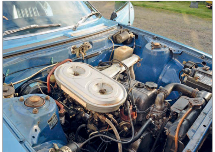
1600 OHV engine is common, with twin carbs.
