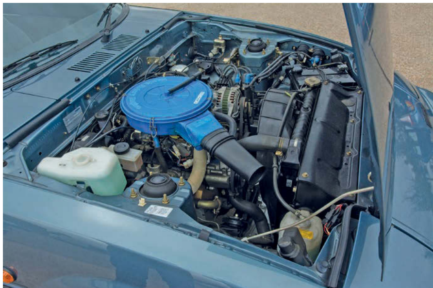
All RX-7s use Mazda's rotary engine family – the 11A or 13B series.
