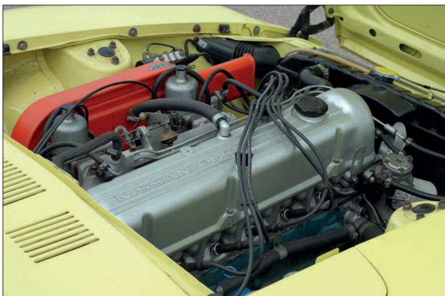
L24 powerplant dominates engine bay. Note Hitachi SU-style carbs.
