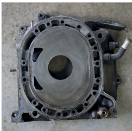
An end plate from an RX-8 – note the inlet and exhaust ports to the left.
