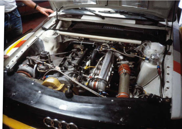
Five-cylinder turbo firepower – the final Sport S1 E2 produced well over 500PS. Photo: Graham Road
