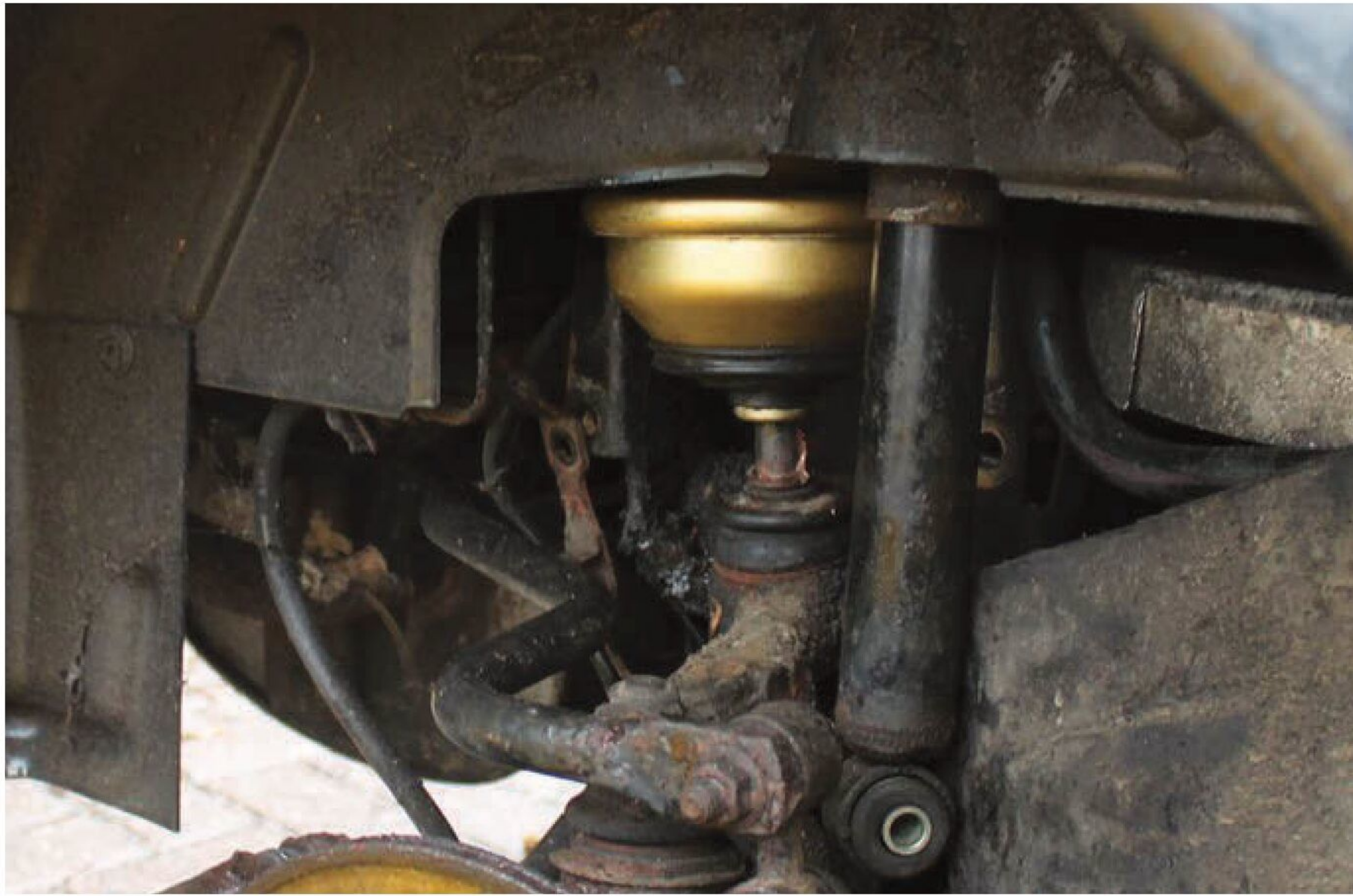
Hydragas spheres tend to have lost their gas by now and need replacing.
