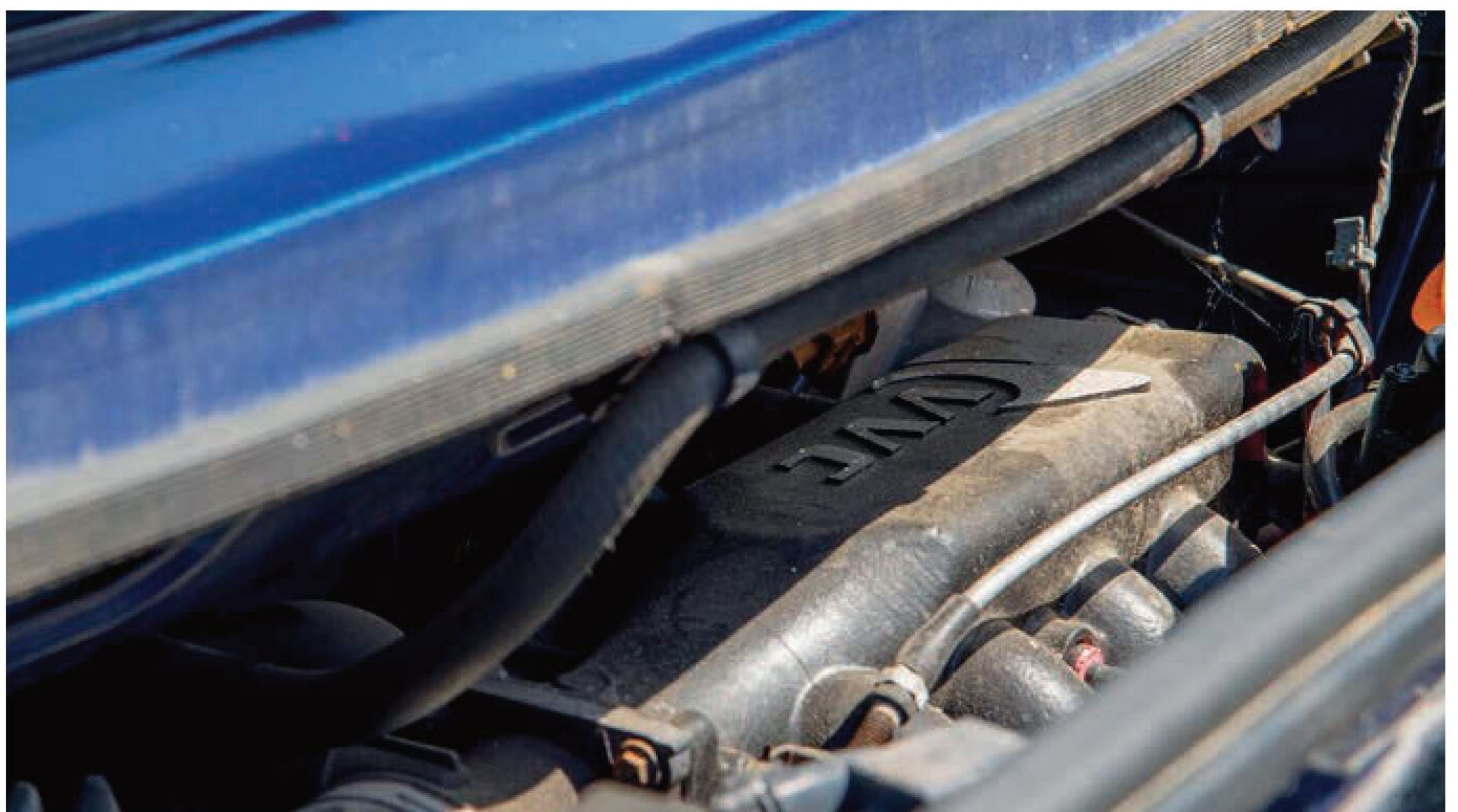
MG's mid-engined layout can make access awkward for anything but basic checks.
