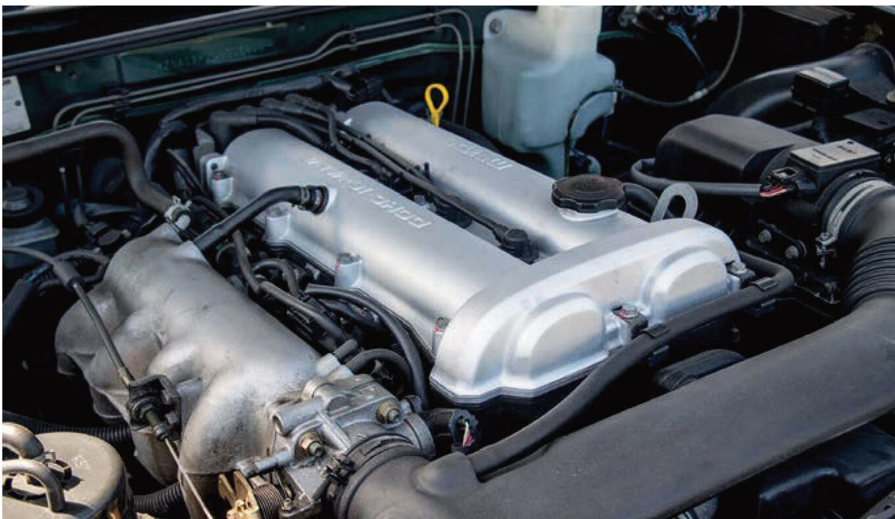
The MX-5's twin-cam engine was derived from the unit in the 323 saloon.
