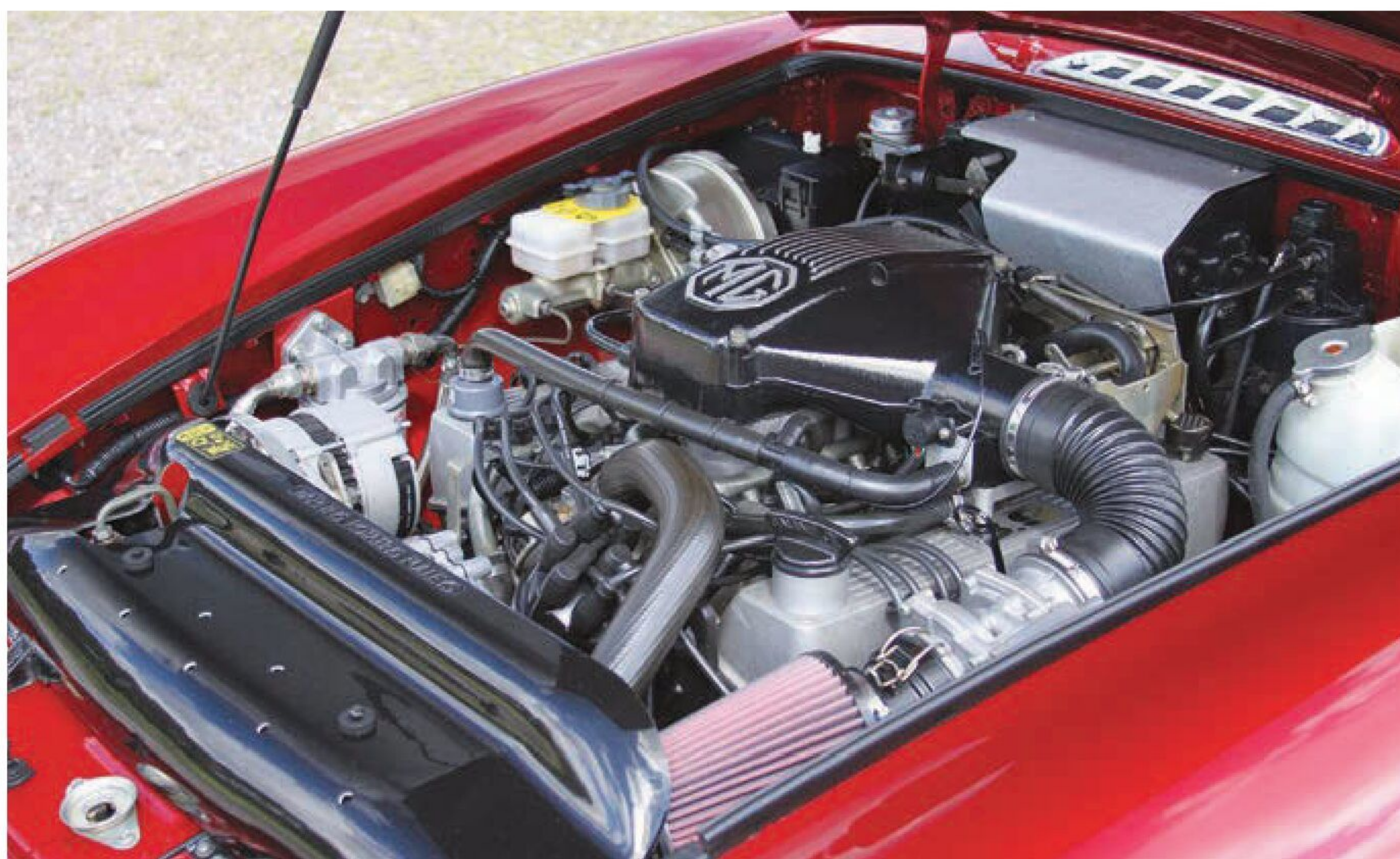
The injected V8 was a tight fit even in the modified MGB shell.
