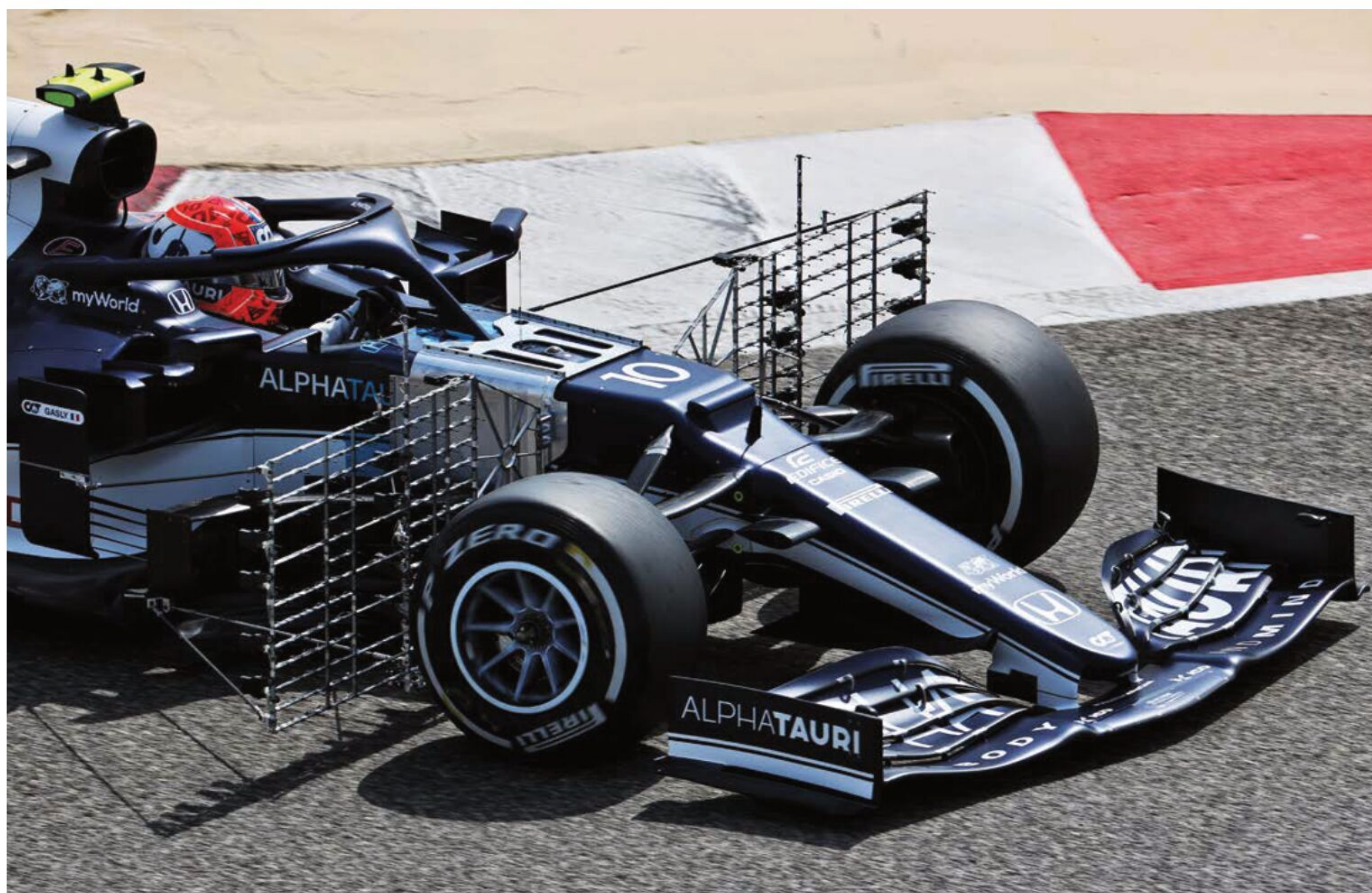
Special instrumentation is fitted to cars at test events. In this case, an array of Kiel probes to correlate laboratory / CFD data
