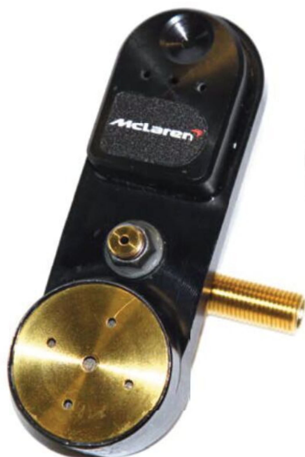
TPMS sensors are mounted to the rim and an infrared element measures the temperature of the underside of the carcass
