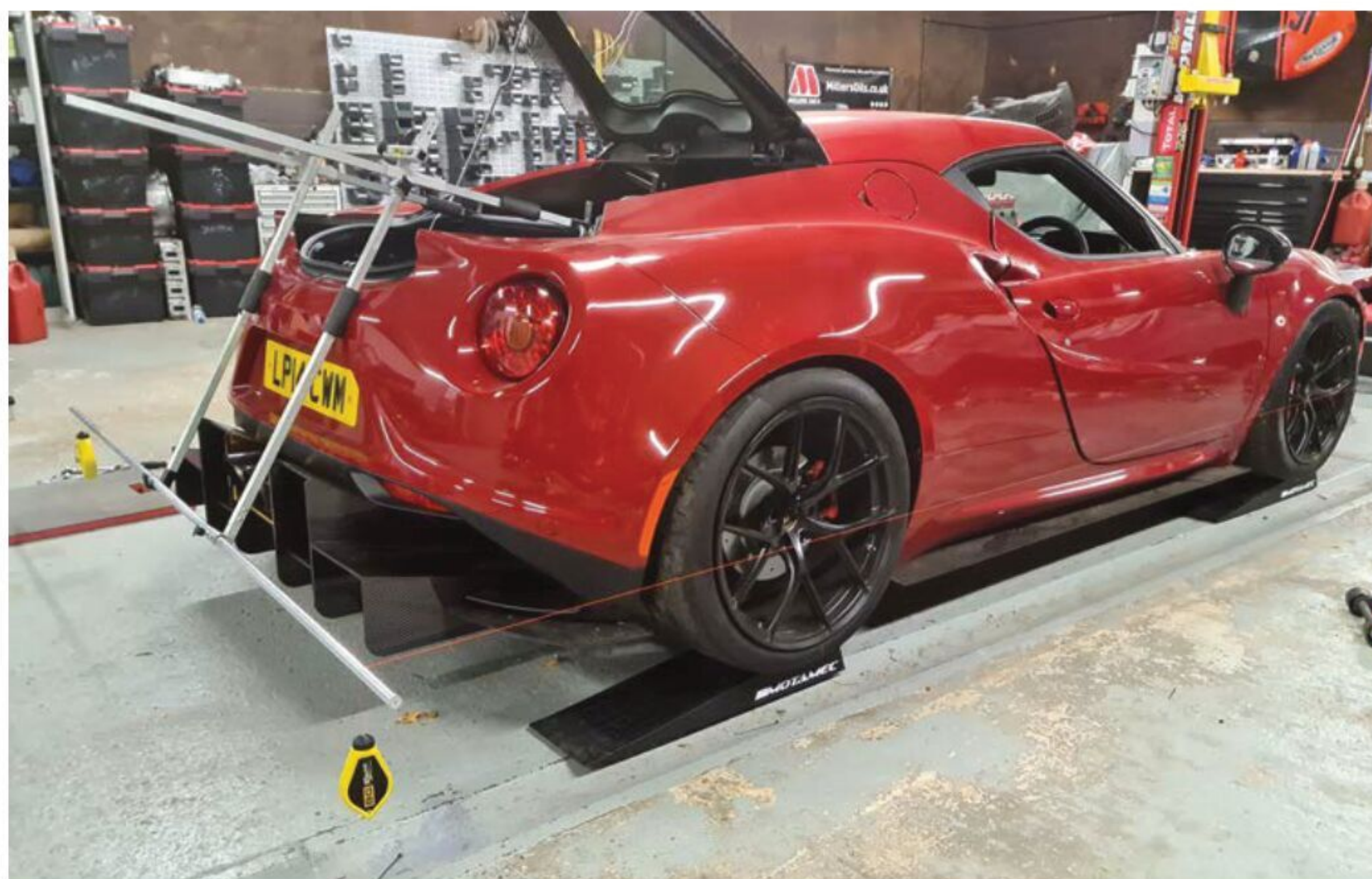
Aside from the calculations, it is imperative to measure the car correctly, and for this there is always the reliable red string
