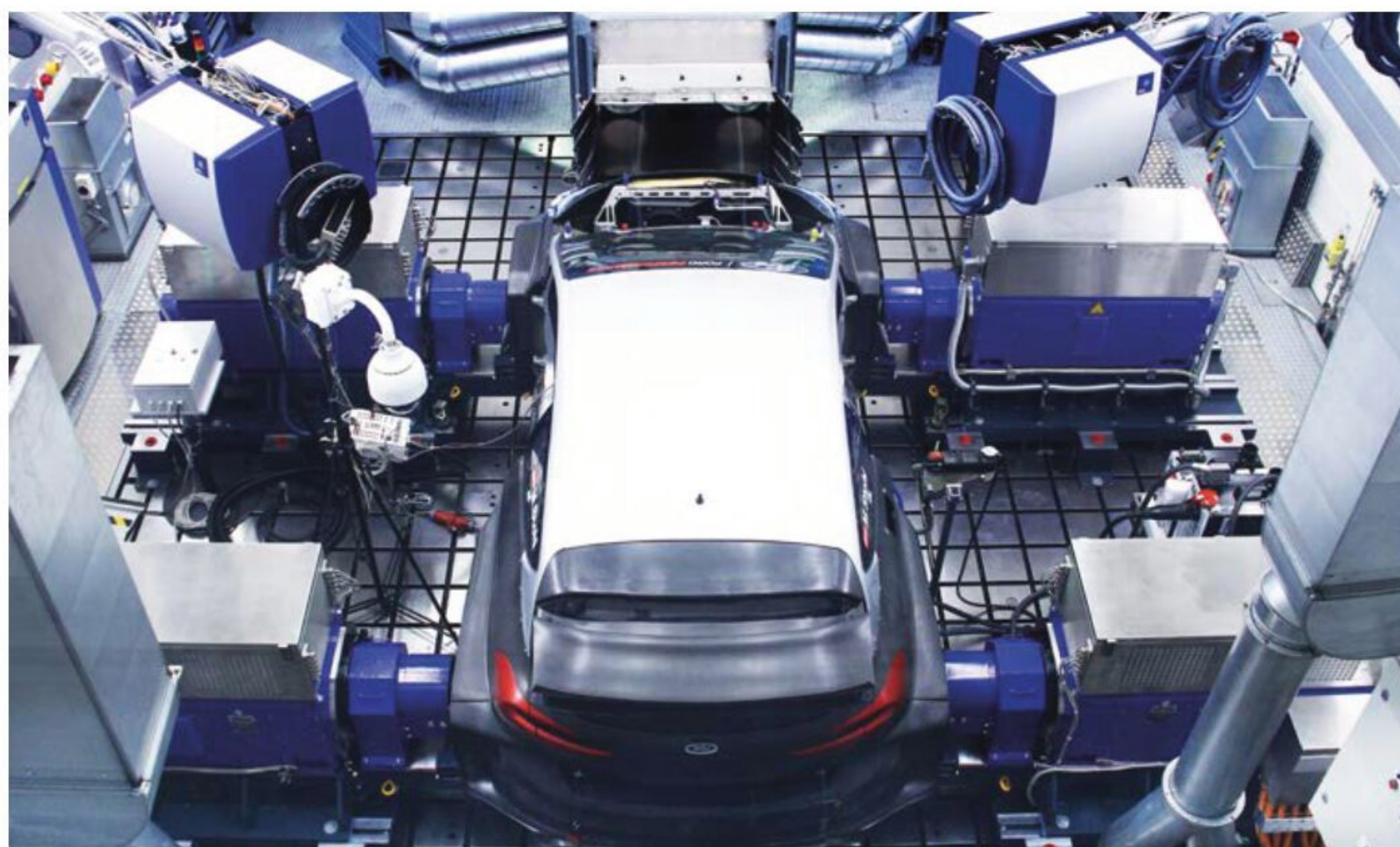
The car on AVL's Full Vehicle Dyno, capable of generating the 800kW needed for Formula 1 and modern EV racecars
