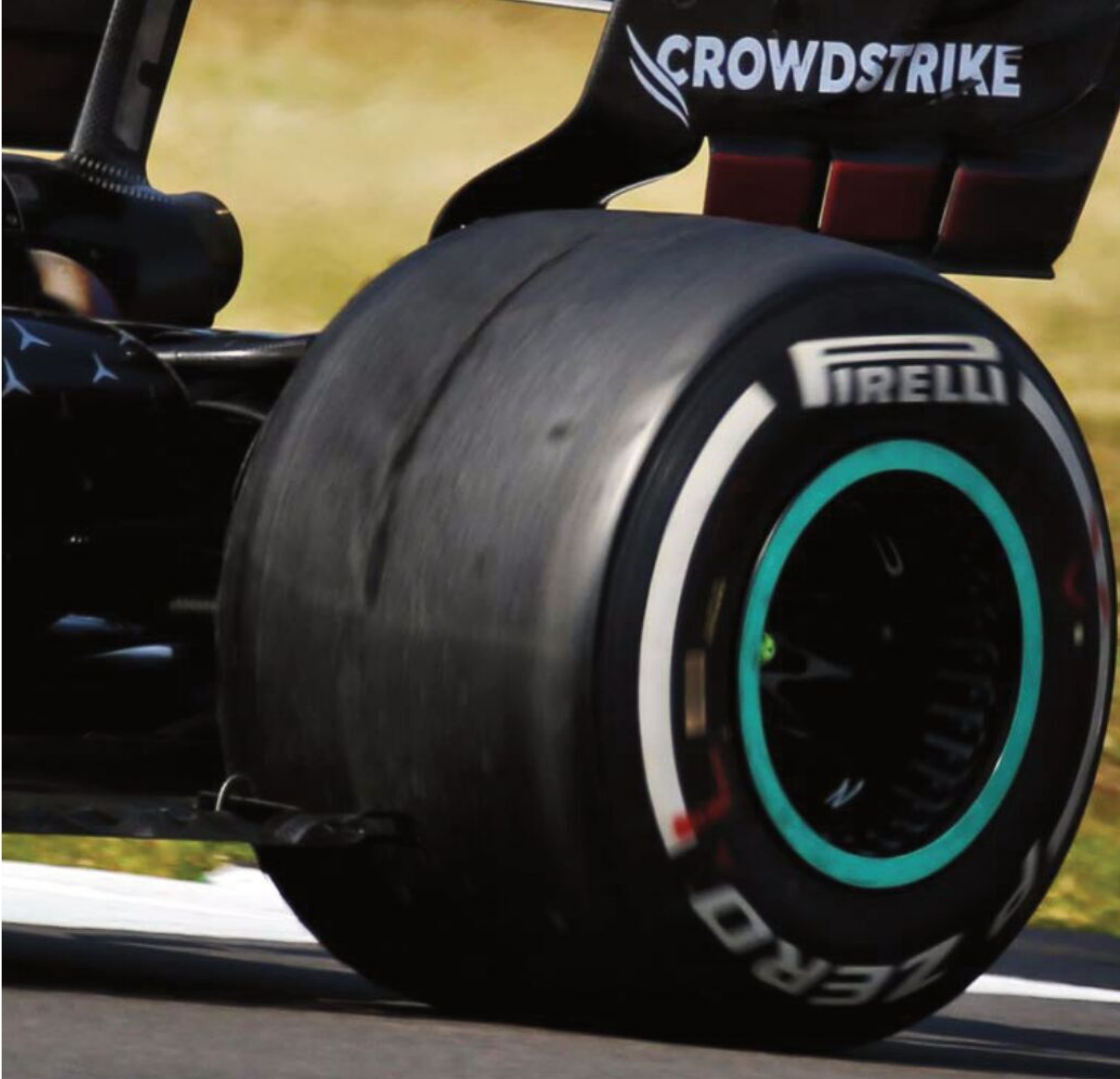
Blistering, where hot spots within the tread form bubbles that explode and rupture the tyre surface, often occurs on the centre of the rear tyres and on the inner shoulder of the fronts as this is where the tyres are hottest during use
