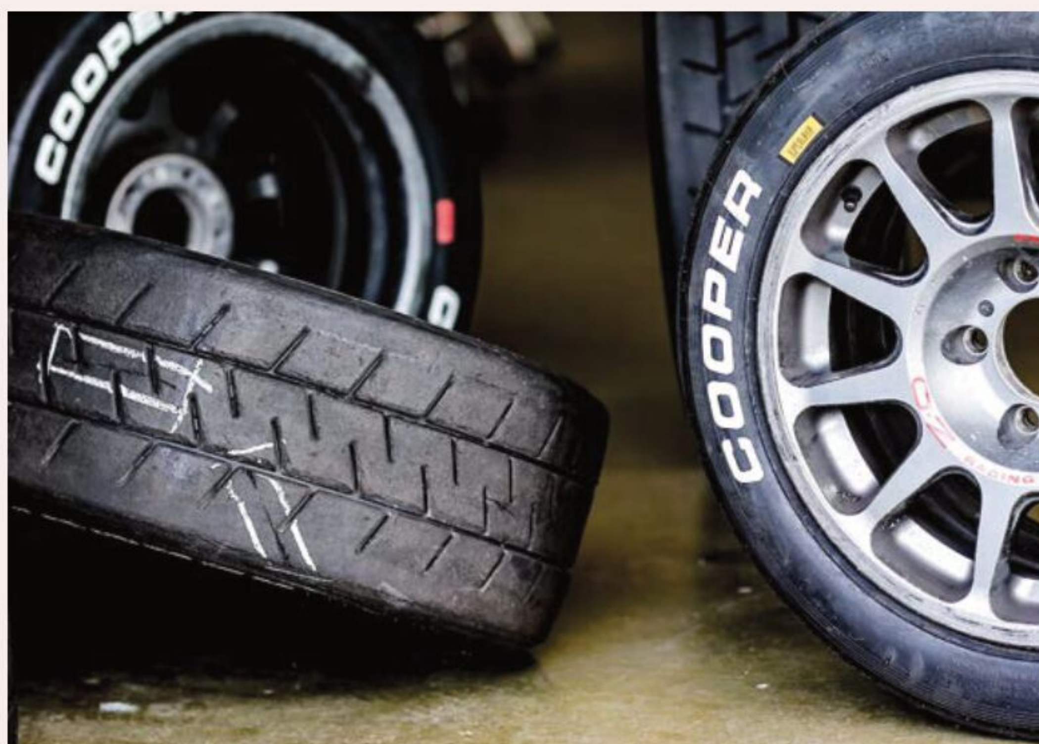
World RX tyres have to work in ambient temperatures between five and 40degC, operating temperatures between 70 and 120+degC and be able to withstand a brutal working regime
