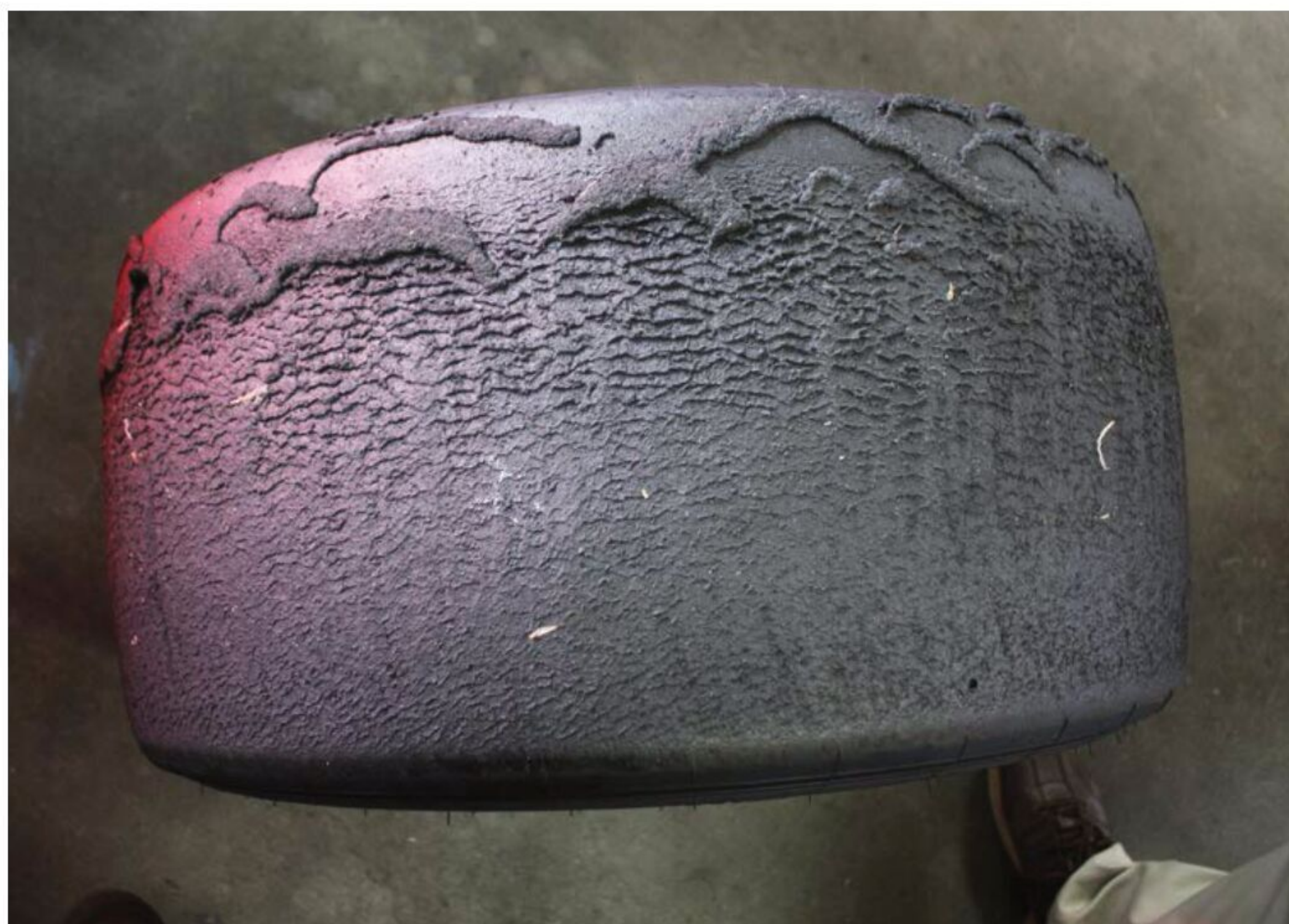
Graining is a common sight in most motorsport categories and indicates the surface of the tyre is overheating. The consequent radial ridges produced reduce the contact patch between tyre and track, reducing available grip
