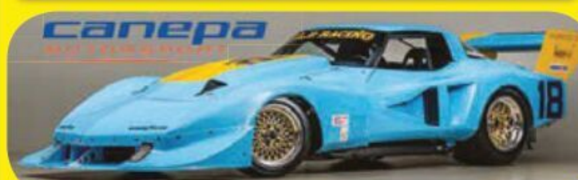
Super Vette, Riley Tube chasis, engines by Lee Muir. Ran Kinsler crossram manifold and Lucas mechanical metering.
