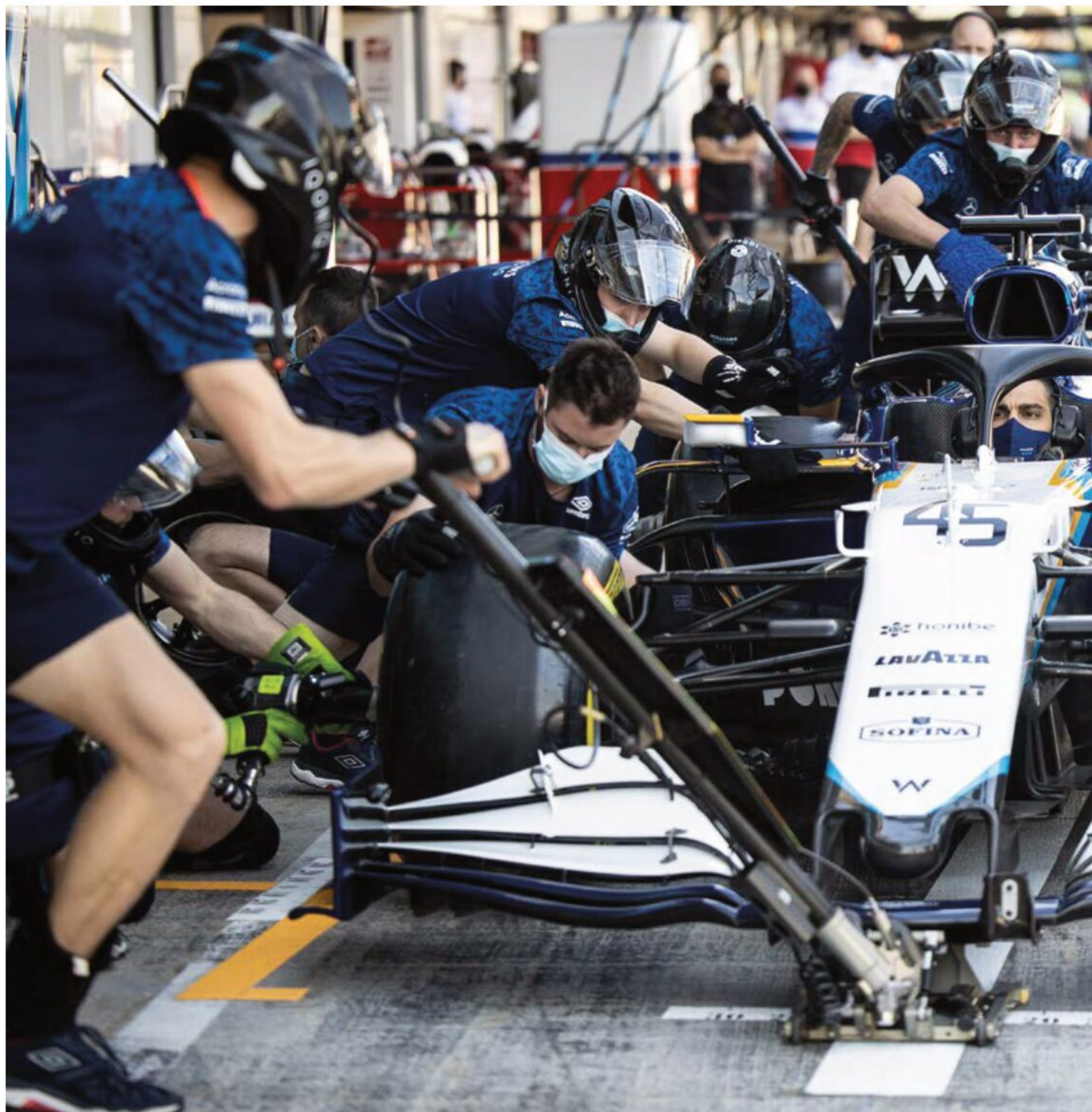
Lifting cars via a manual or on-board jacking system is important in the garage and on pit lane
