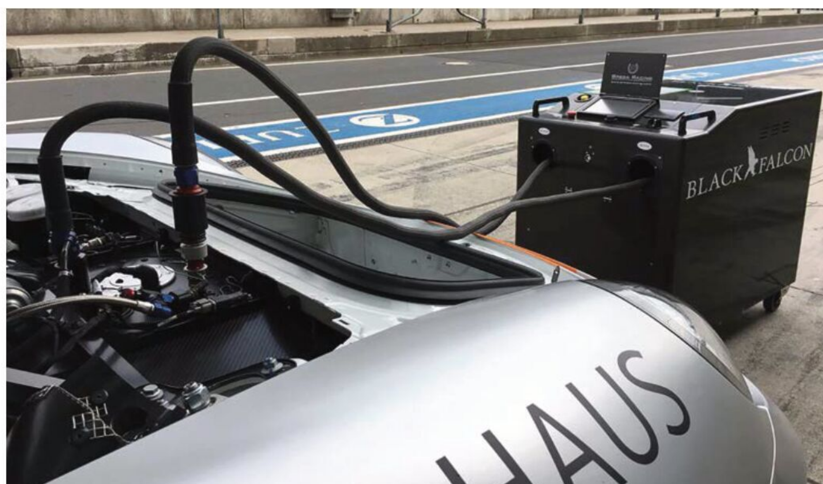
Today, computer-controlled bowsers can automatically transfer fuel from the storage barrels in the pits to the car's fuel tank
