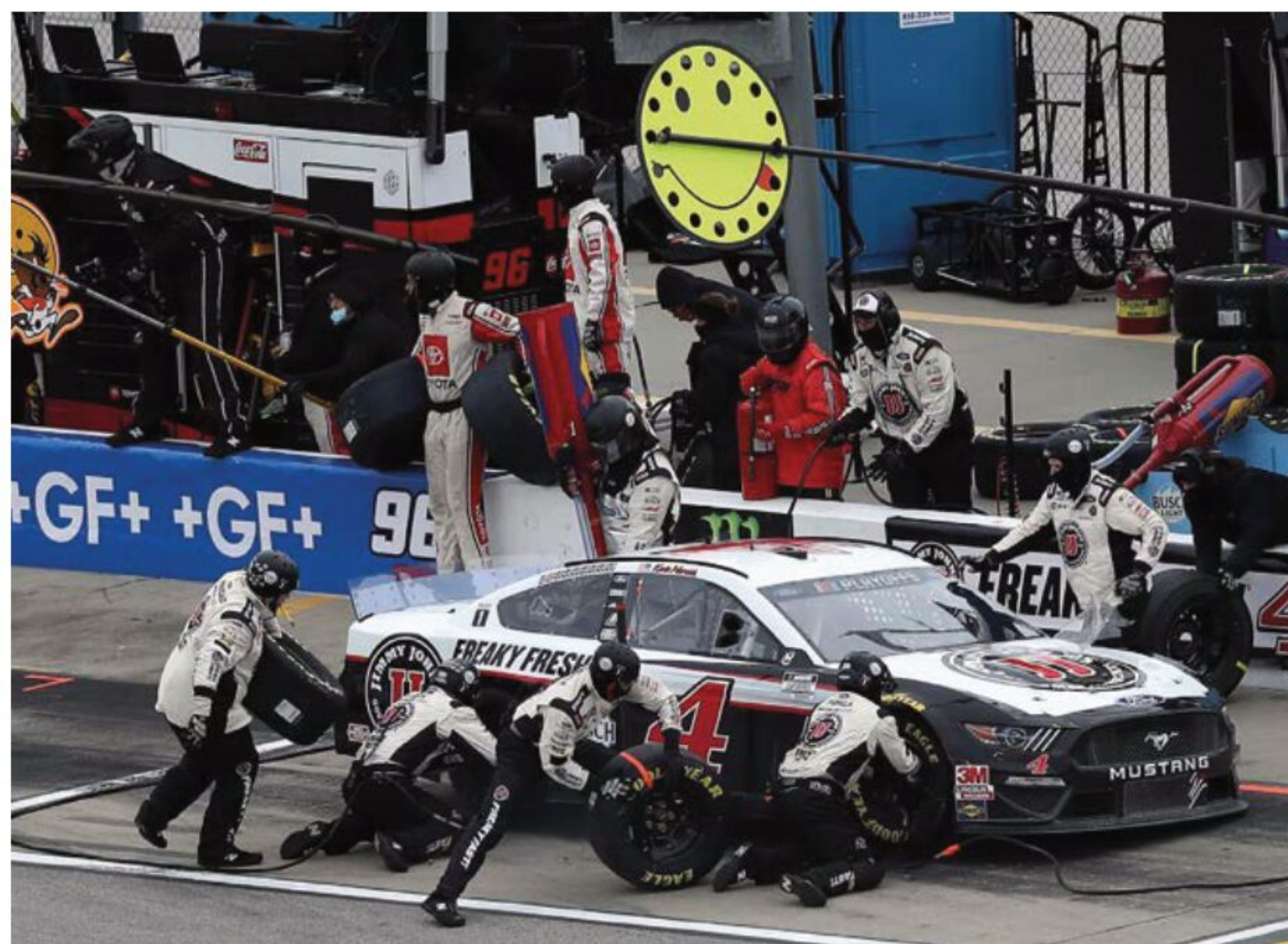
A modern day NASCAR pit stop. The refuelling operators have to physically manoeuvre 50kg dump cans
