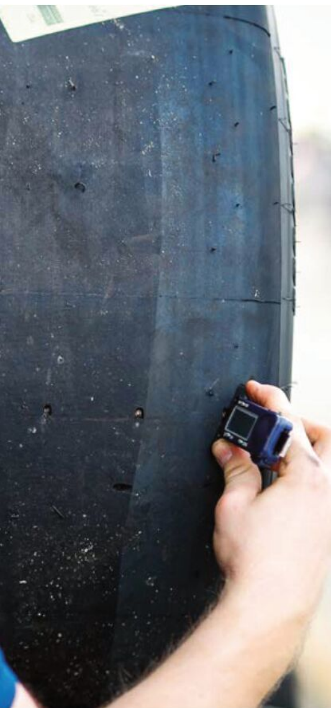
The result is a wear profile that illustrates the amount of tyre consumed at each TWI, for each of the four tyres on the racecar. The wear pattern of four different sets of tyres are shown here
