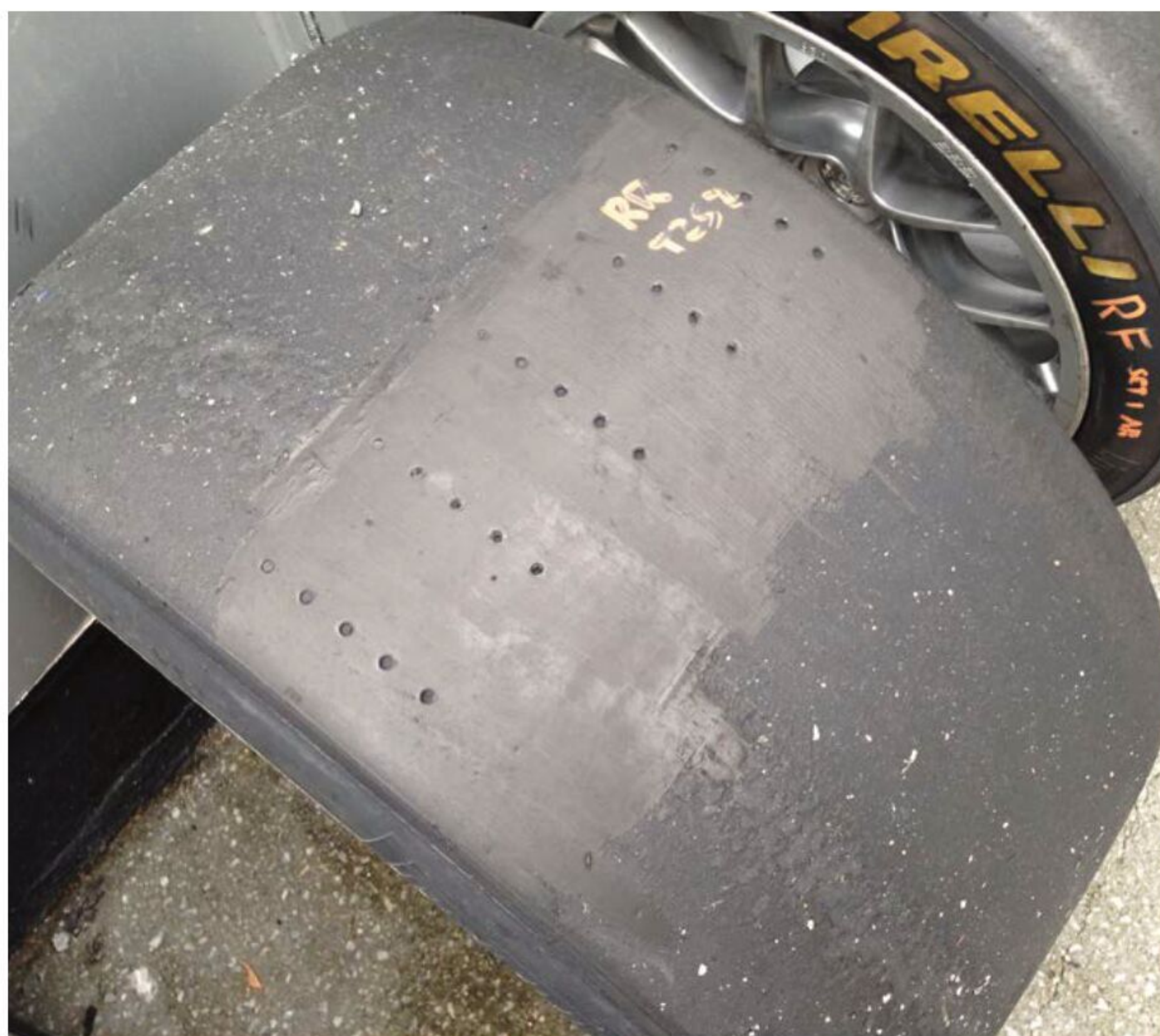
Tyres have a series of tread wear indicators (TWI), which are different depth holes used to measure the wear of the tyre. But before they can be ‘read’, any pick up has to be heated and scraped off
