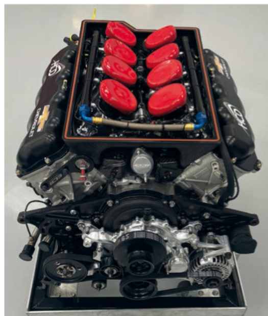
Remarkably little was changed from Cup spec, just a tweak of the oiling system, a different cam and a new set of pistons and rings
