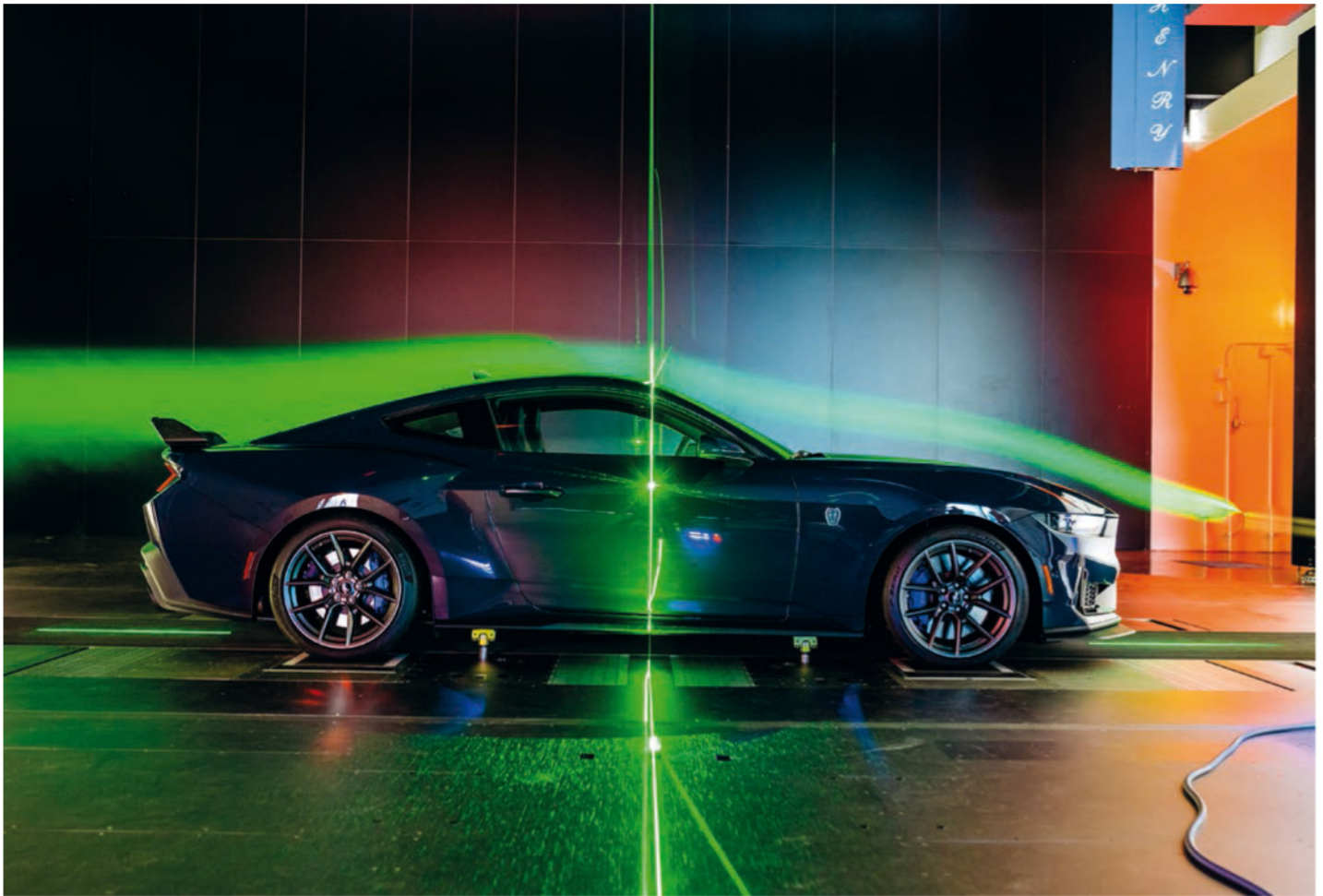
Ford was so convinced by the Windshear technology that it developed its own rolling road wind tunnel, which is helpful in the development of electric vehicles, as well as combustion cars
