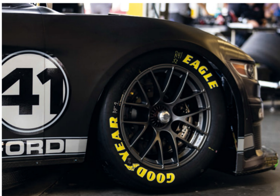
Side skirts were removed, and the Next Gen cars have a full-length, aerodynamically-driven, carbon fibre underbody, plus 18in rims
