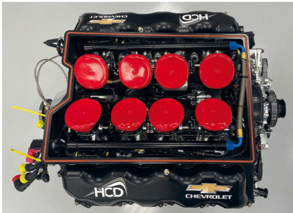
Remarkably little was changed from Cup spec, just a tweak of the oiling system, a different cam and a new set of pistons and rings
