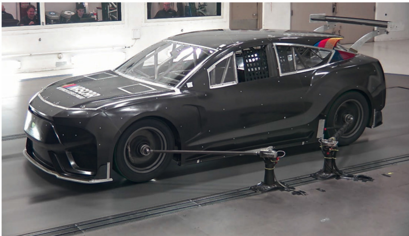
With the CUV-style body shape, aerodynamic performance was a concern, so the prototype was investigated at Windshear in North Carolina and at Stellantis' wind tunnel for its yaw angle capability
