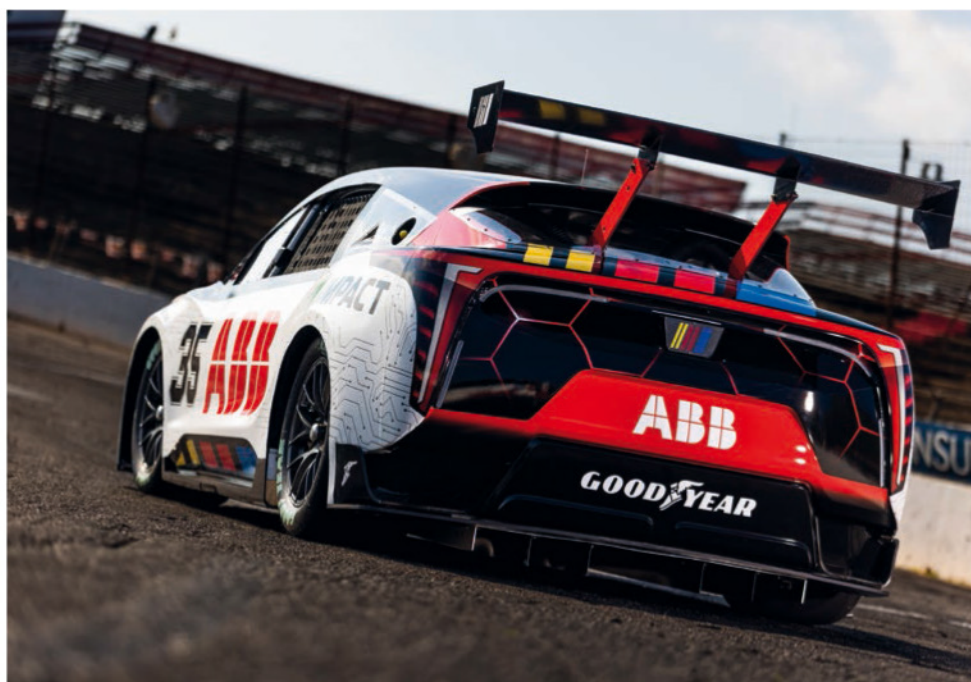
A rear wing was considered more effective than a traditional NASCAR spoiler, a major departure for the sport's aerodynamic concept
