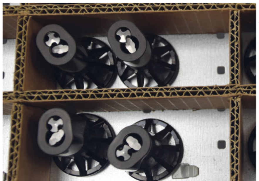
These delightful little screw pumps, which Schirle describes as 'mini superchargers', are at the heart of the Cobra pump
