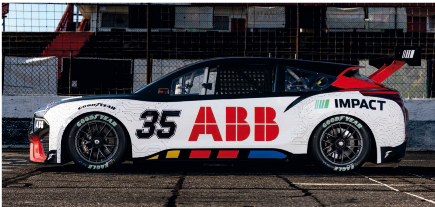
The design team says it reflected on current automotive purchasing trends in the US so, while the EV uses the Next Gen chassis, the body design is based on a generic Crossover Utility Vehicle (CUV)
