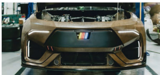
BComp's flax fibre bodywork was tested, possibly for future application
