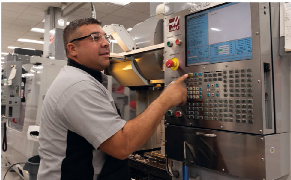
Starting from raw block castings bought in from General Motors, all machining tasks are done in-house for tight quality control
