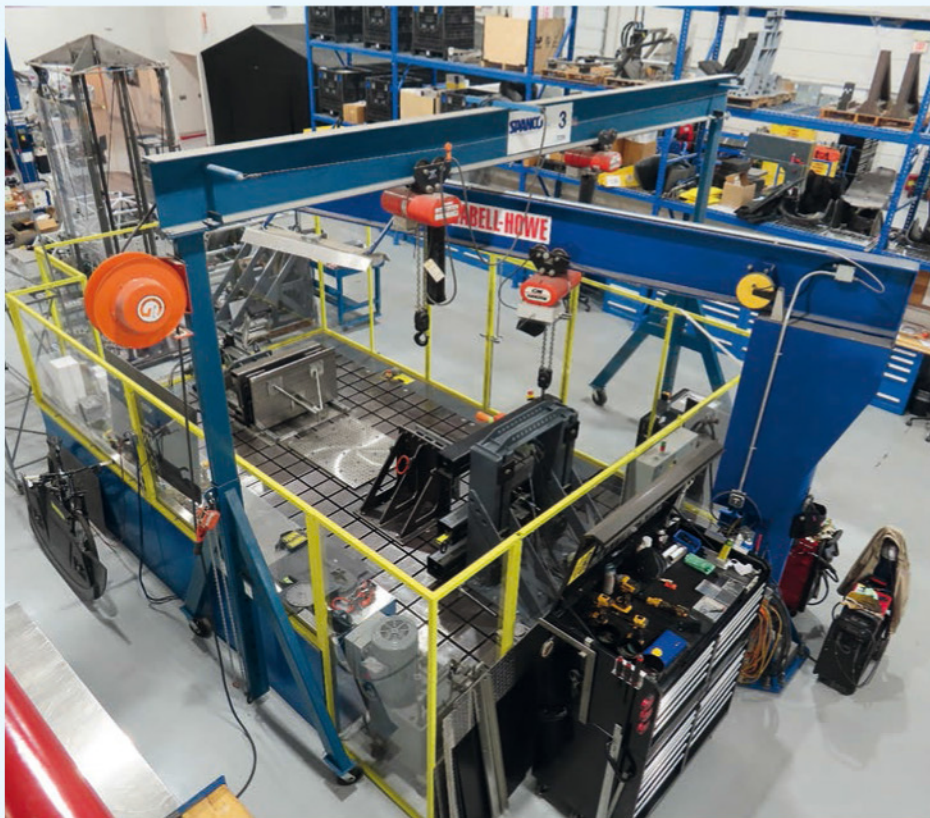
Much of the work that takes place at the R&D Center is about improving safety. Shown here is the safety department's quasi-static testing rig, which is used for assessing anchorages, seat deformation and more. Full-scale vehicle crash testing and sled testing is conducted off-site
