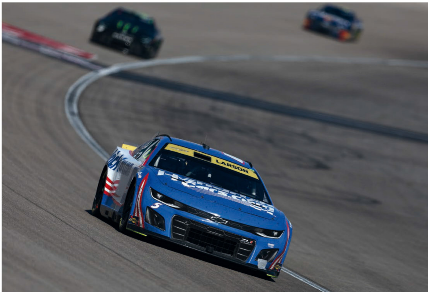
The new, coupé body shape behaves very differently to the Gen 6 car, but the aero modifications made underneath mean drivers in the pack struggle to reel in cars running in clean air at the front
