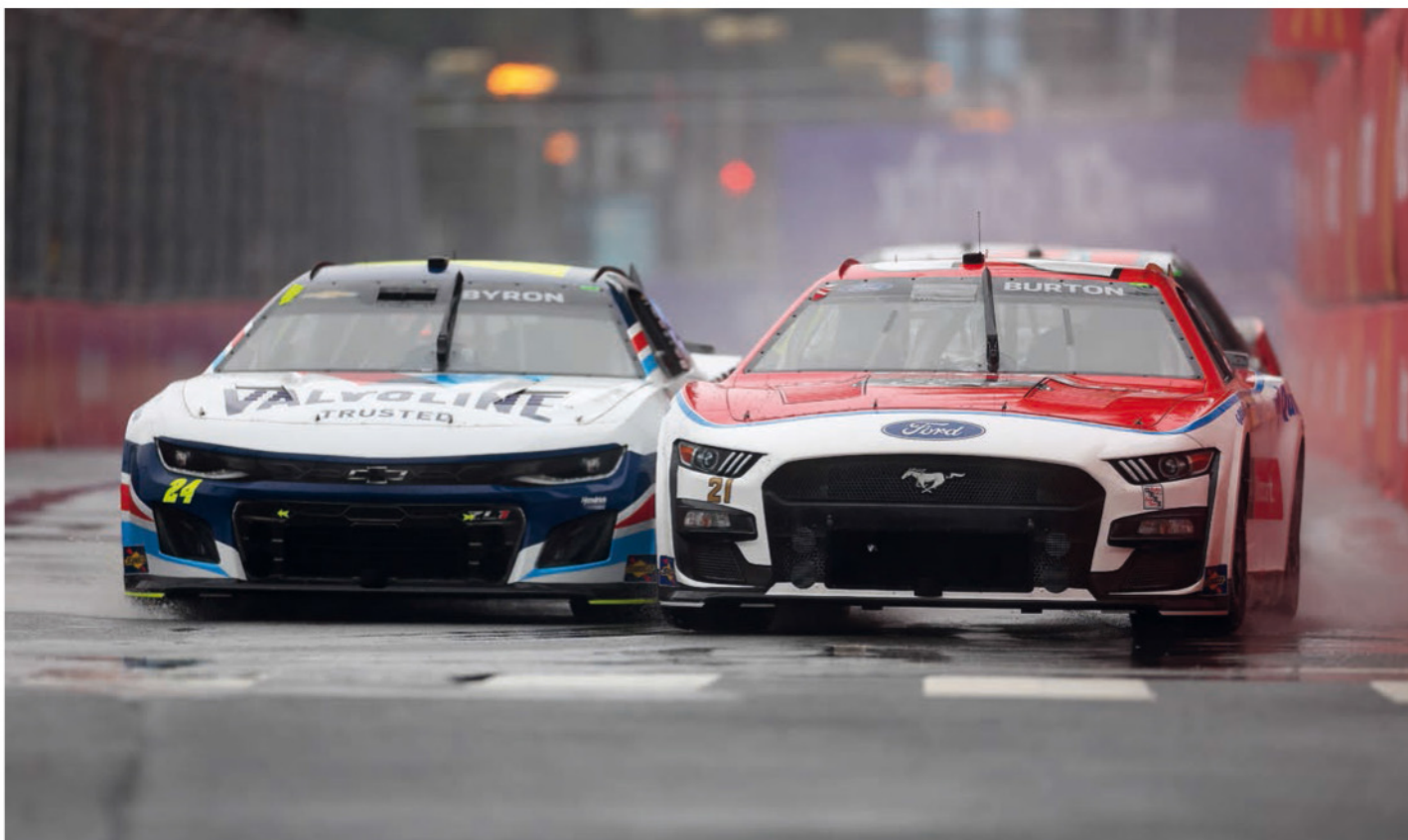
NASCAR runs in the wet with a package that includes wipers, rain lights and flaps, along with appropriate Goodyear tyres. This became available for 2023, on some ovals as well as road courses
