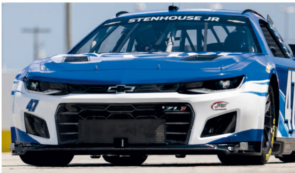
In achieving the goal of matching the downforce and aero balance of the outgoing Gen 6 car, the front splitter played a crucial part
