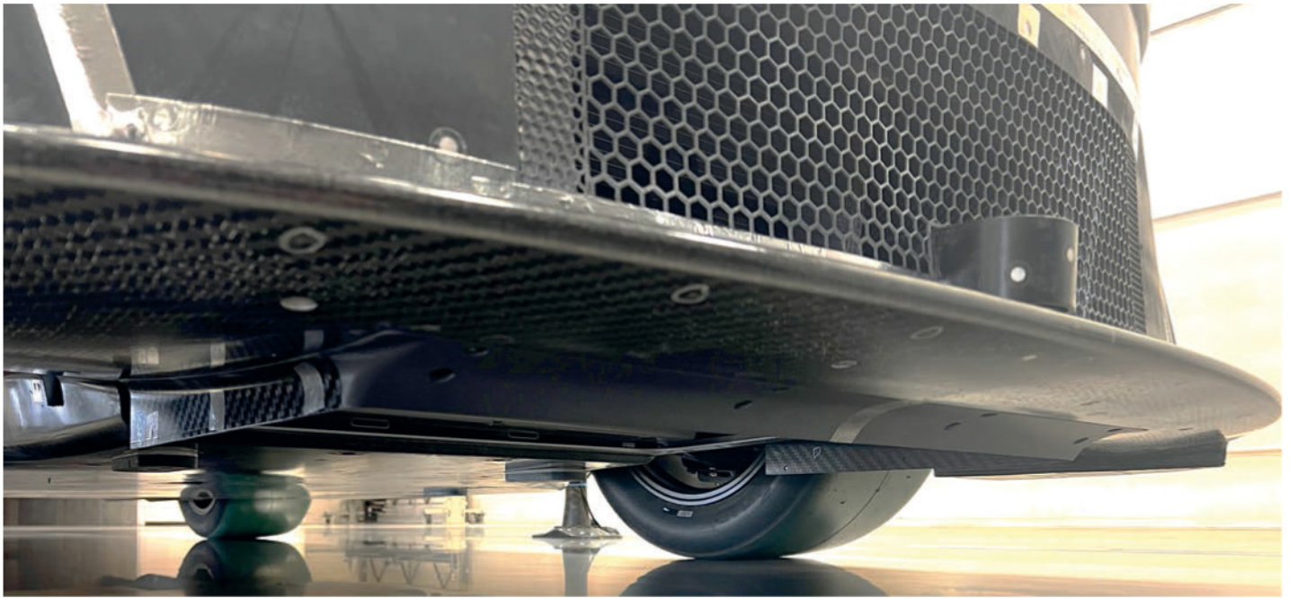
The solution to improving fan engagement with the racing on NASCAR's short tracks and road courses is the so-called up / down splitter, seen here installed on the aero test car at Windshear
