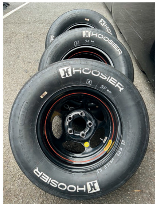
Cars run on a set of 330 / 700 R15 slick tyres from Hoosier, which replaced General Tire as the NASCAR Euro Series supplier in 2021
