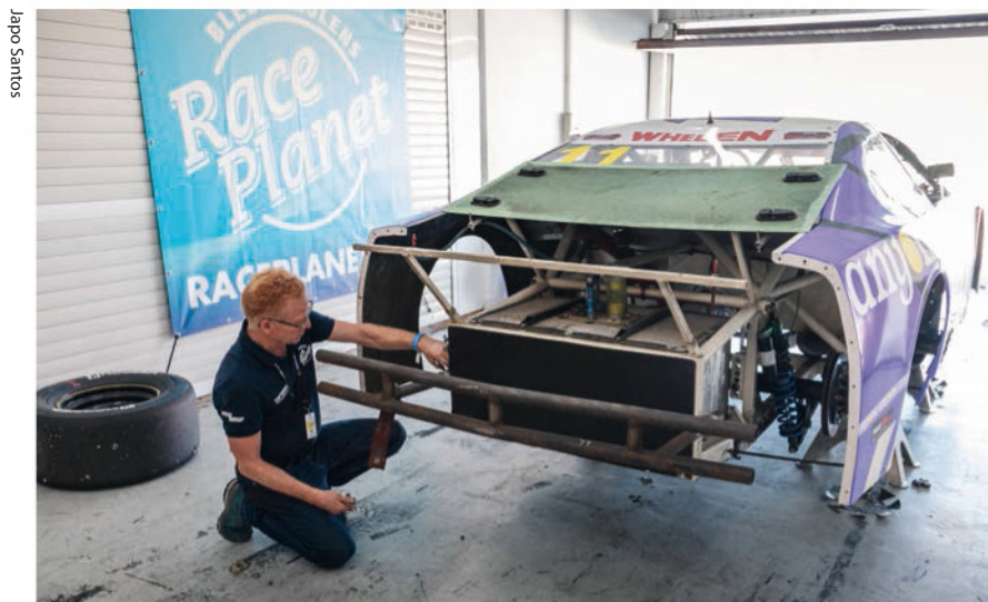
Team FJ in France assembles the chassis, which is homologated as EuroNASCAR-RC01 and has been in use since 2009
