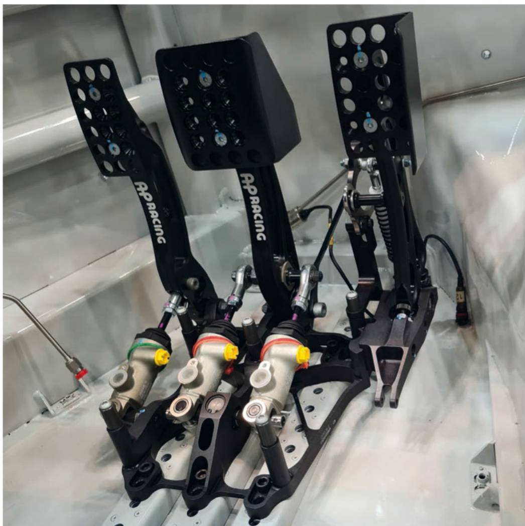
AP's Next Gen pedal box offers five different pedal ratios and a choice of 10 bore sizes on the brake cylinder so teams can tune their brake system
