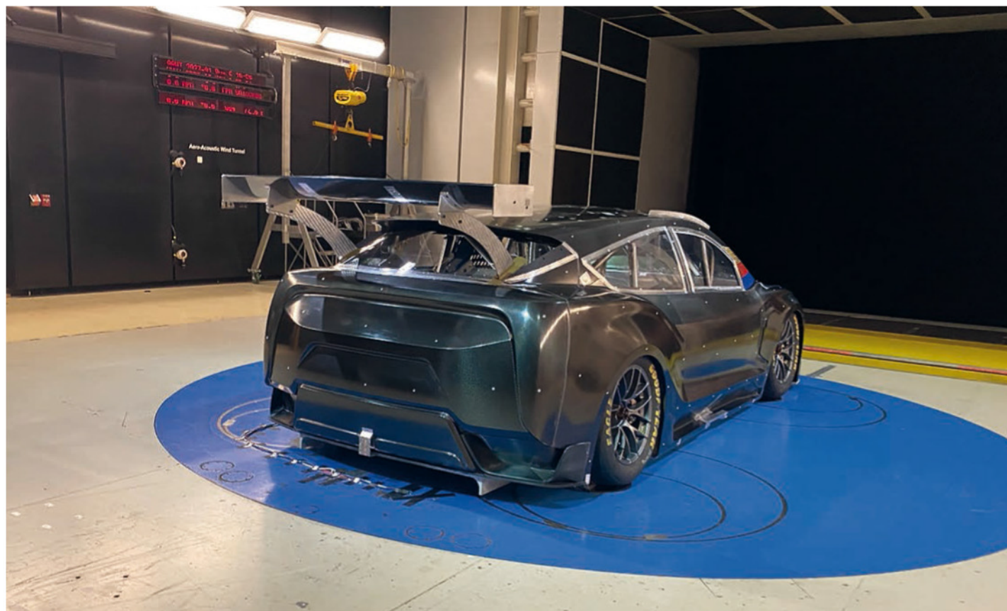
The aero test mule undergoing investigations at Chrysler headquarters in Michigan. Engineers were surprised to find the vehicle shape performed better than expected in the lift-off safety tests
