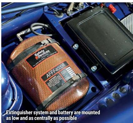
Extinguisher system and battery are mounted as low and as centrally as possible
