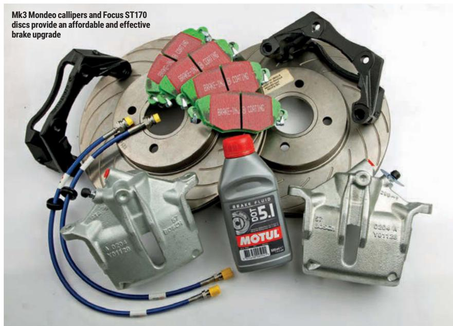
swap to Mondeo Mk3 callipers and Focus ST170 (four-stud) 300mm discs, which are a direct fit – needing only 3mm spacers and slightly longer bolts. The only drawback is they don't fit behind ST24 16in alloys; ST200 17s go on just fine.
