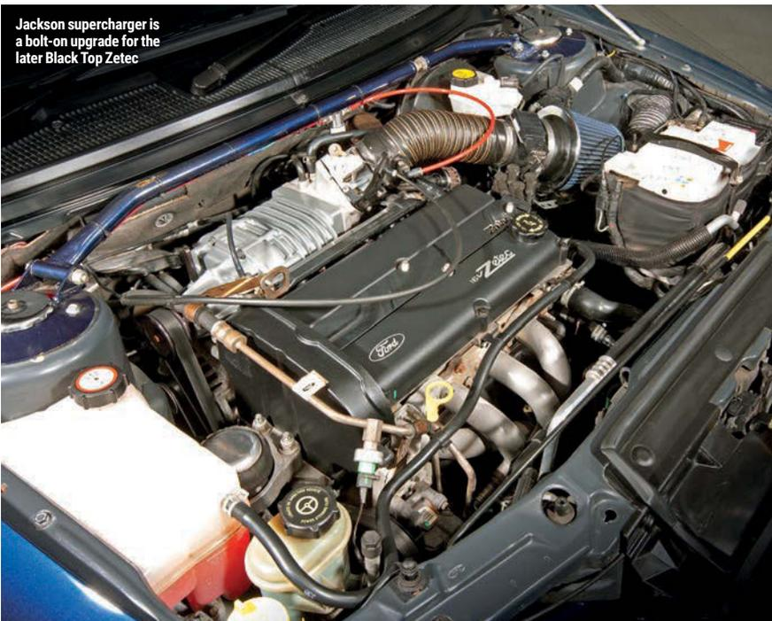
Jackson supercharger is a bolt-on upgrade for the later Black Top Zetec
