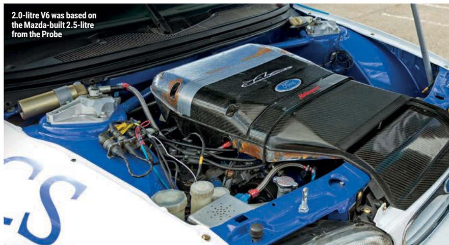
2.0-litre V6 was based on the Mazda-built 2.5-litre from the Probe
