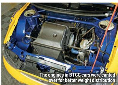
The engines in BTCC cars were cantilevered over for better weight distribution
