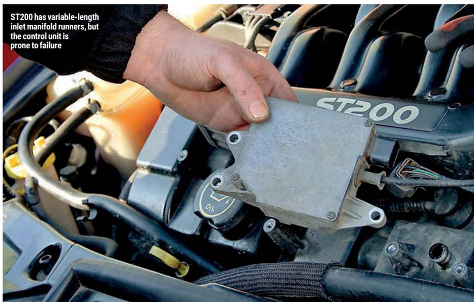
ST200 has variable-length inlet manifold runners, but the control unit is prone to failure
