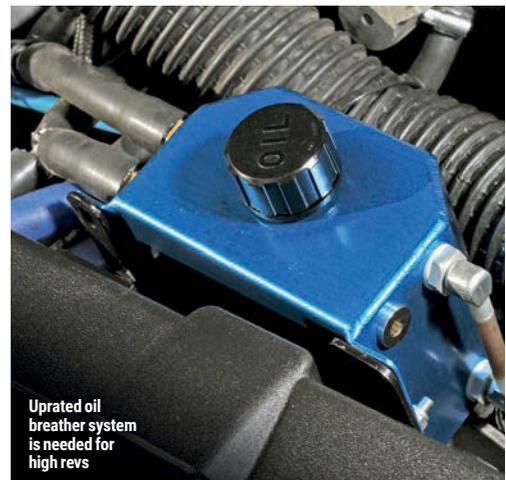
Uprated oil breather system is needed for high revs
