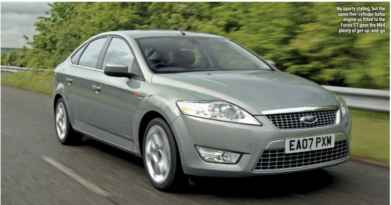
No sporty styling, but the same five-cylinder turbo engine as fitted to the Focus ST gave the Mk4 plenty of get-up-and-go
