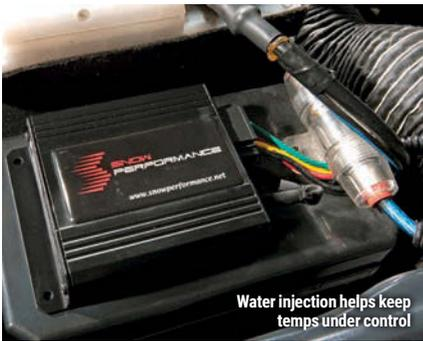
Water injection helps keep temps under control
