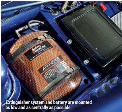
Extinguisher system and battery are mounted as low and as centrally as possible
