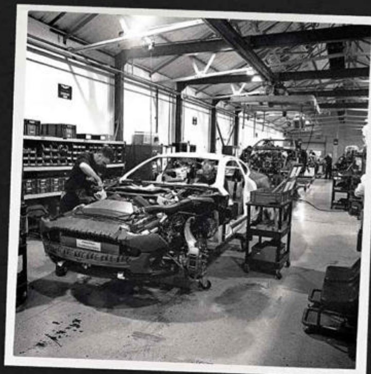
Left Hand-finishing a Vanquish body before it progressed to the paint shop. Each Vanquish carried a plaque saying 'Handbuilt in England' together with the name of the person who carried out the final inspection, and the engine number – a nice echo of earlier Astons, whose V8 engines carried the name of the engine-builder
