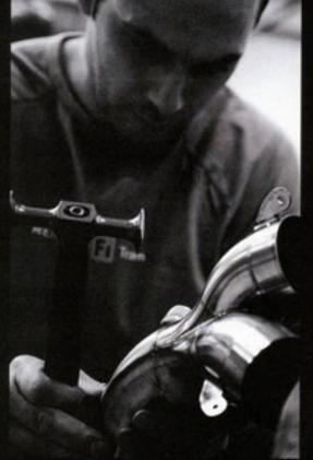
intercoolers and more — to today's smaller range of components. Renault still employ eight full-time fabricators, but they're part of a dying breed in F1. Any new recruit needs about five years working as an apprentice to truly master the skills — along with exhausts, they produce radiator housings and many of the custom objects an F1 team needs, like the pitwall telemetry housing. After all, you can't just pop down to B&Q and order one.
