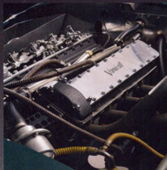
The powerful 2.5ltr Vanwall engine pumped out up to 285bhp at 7,500rpm, depending on what fuel was in the tank
