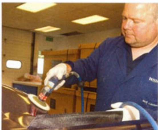
Before undergoing the arduous-sounding 'non-destructive test' the wing is checked for quality and then buffed to a shine
