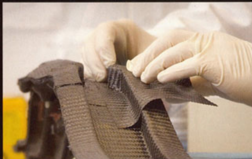
A wing spar starts out as many small sheets of carbon fibre, cut from a giant 50m roll and stuck into place on the mould
