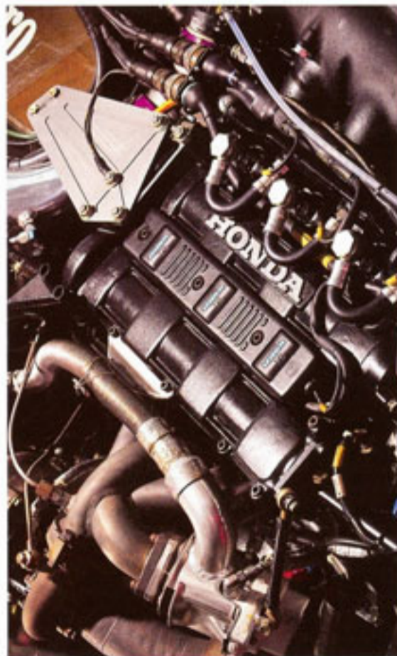
The Honda V6 turbo RA168-E powered the MP4/4. The Lotus 100T couldn't get near McLaren that year, despite using the same unit
