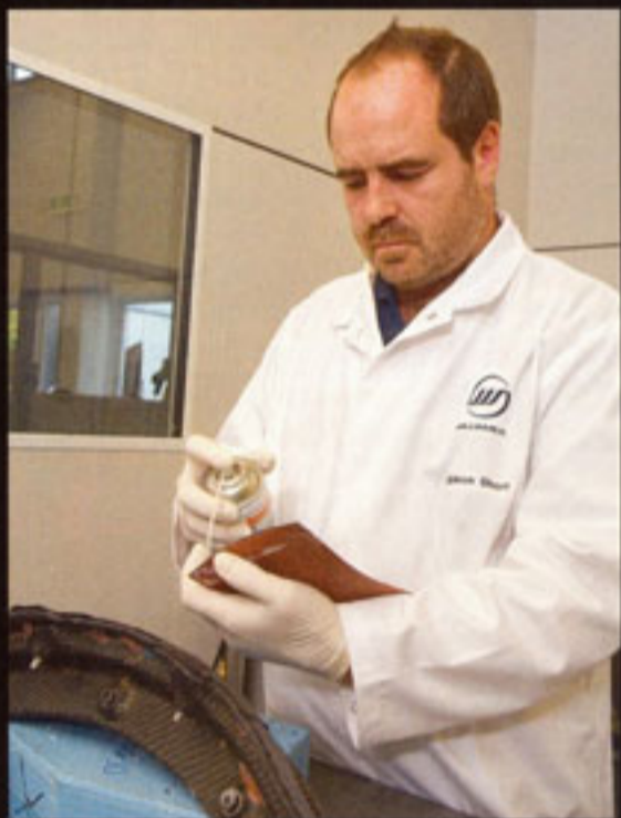
A wing spar starts out as many small sheets of carbon fibre, cut from a giant 50m roll and stuck into place on the mould
