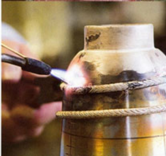
The trophies start out as a circular plate, gradually honed into a cup on a lathe. The constructors' (above left) has 10 sides; each trophy has an adjustable base (below left) so the most recent winner faces the front
