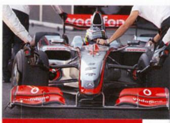
What? Different front wing configurations Where? Found on the McLaren, BMW and Williams What for? New regulations for 2009 state that front wings must be lower and wider. The intention is to improve cars' ability to overtake next year
