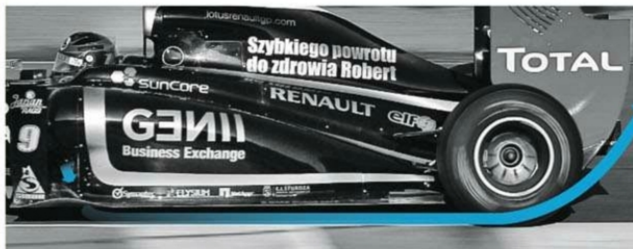
The exhaust plume travels the length of the floor to enter and energise the diffuser at the rear
