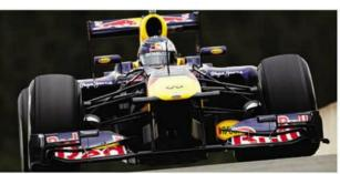
As well as making gains to the overall aero package of a car, you're making aero packages for specific races. Monaco requires a unique high downforce solution, while the long straights of Monza need the exact opposite and the fast sweeps of Silverstone require a mix of aero grip and straight-line speed.
