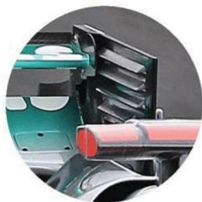
This slot in the rear-wing endplate is exposed when DRS is activated, and stalls the wing
