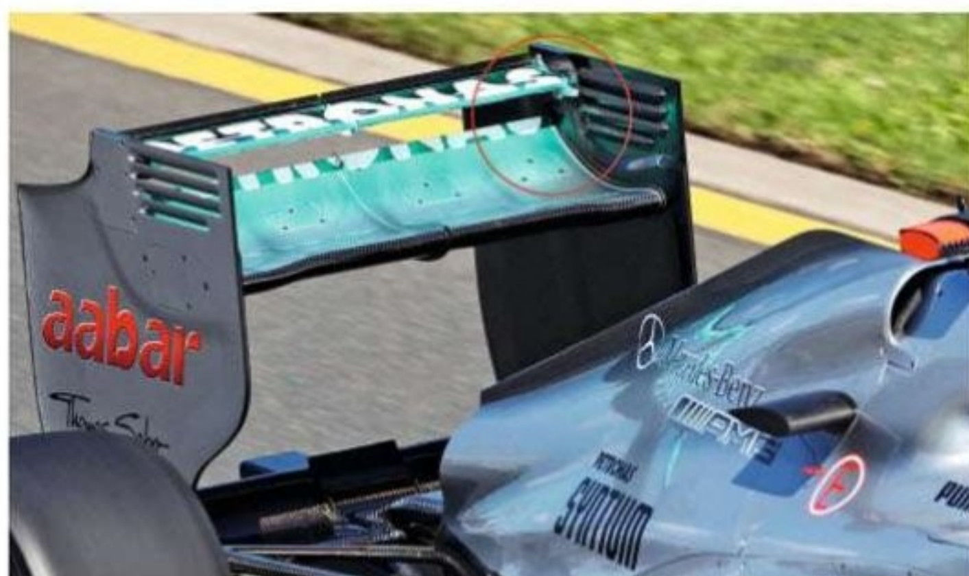
Mercedes' double DRS has a hole in the rear-wing endplate to boost speed
