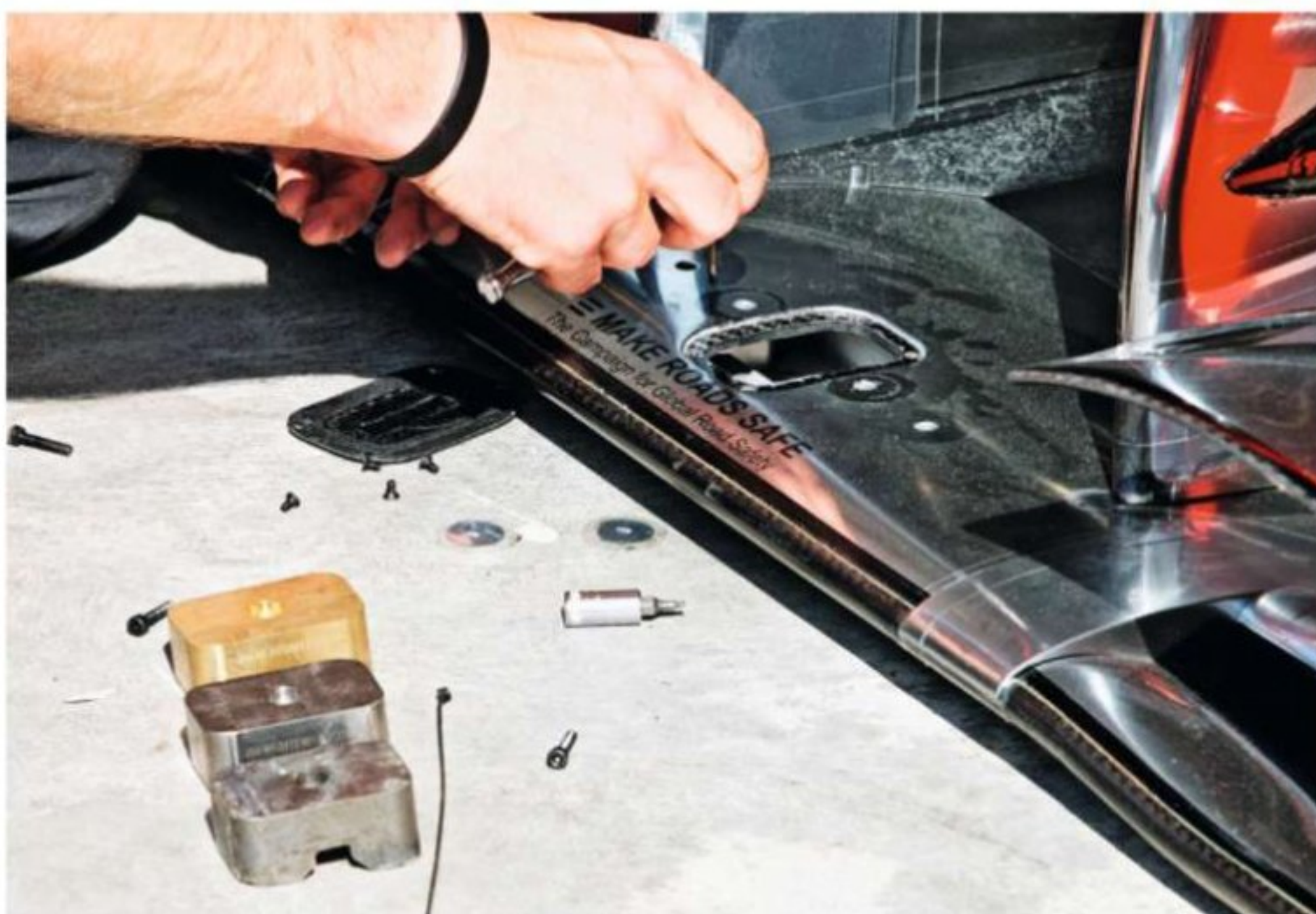
Ballast (usually made from tungsten-based alloys in F1) is added to a McLaren at the 2010 Turkish GP
