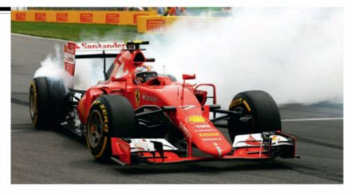
'Start maps' set clutch position and engine demand on the first lap after the race start or a pitstop. They make it harder to control the throttle, which may have caused Kimi Raikkonen's spin in Montréal (right)
