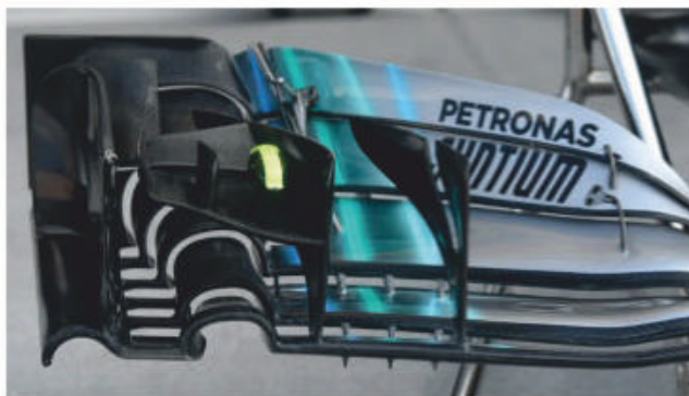
The intricate front wing on last year's Mercedes W09 featured tiny wings to redirect airflow – but the new rules will mean a clean slate for 2019
