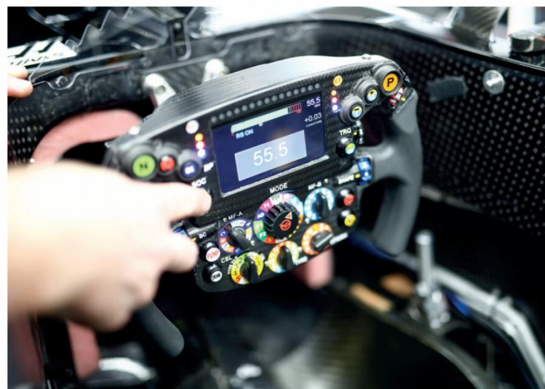
Setting changes can be made mechanically (top) or electronically via the steering wheel (bottom)
