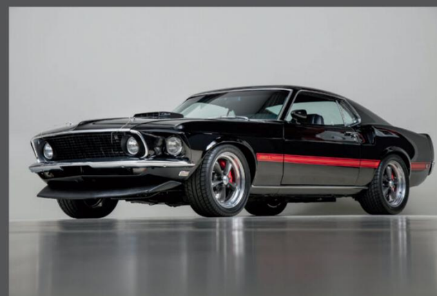
1969 Ford Mustang Mach I No-expense spared “restomod” by Canepa. Original Cobra Jet 428 engine upgraded to 490hp, 517lbs/ft torque. Tremec 5-speed manual trans, modern suspension/brake systems. Vintage Air A/C system.
