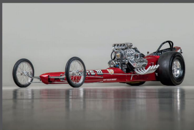
1964 Fuller Roberts Starlite III Owned and driven by Chuck Griffith . Built by Kent Fuller , body by Arnie Roberts . 2,000+hp, nitromethane 400ci Chrysler Hemi Supercharged V8. Quarter mile time 7.5+ seconds - 200+mph.
