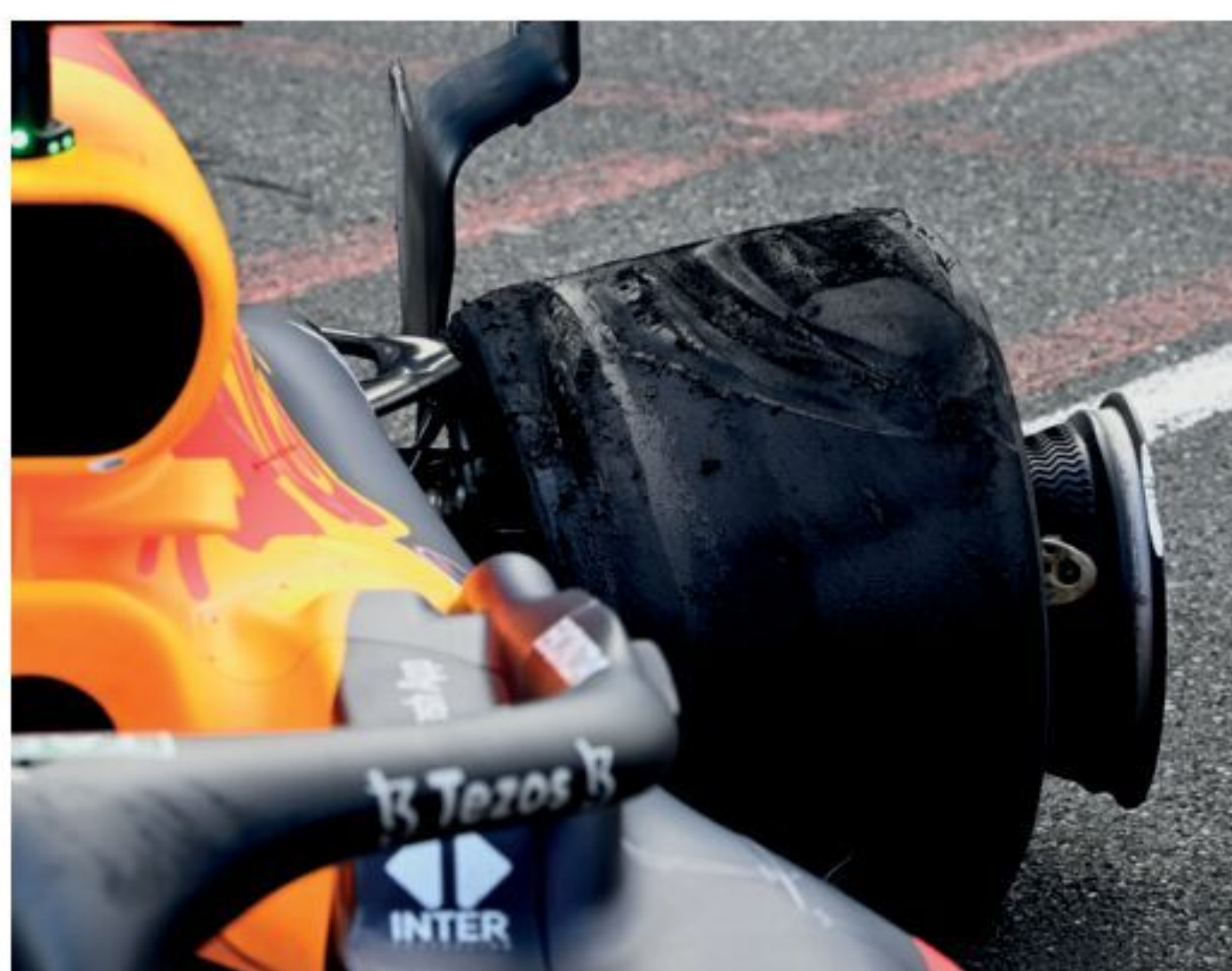
The damage to Verstappen's tyre that caused his accident in Baku led to a detailed investigation by Pirelli
