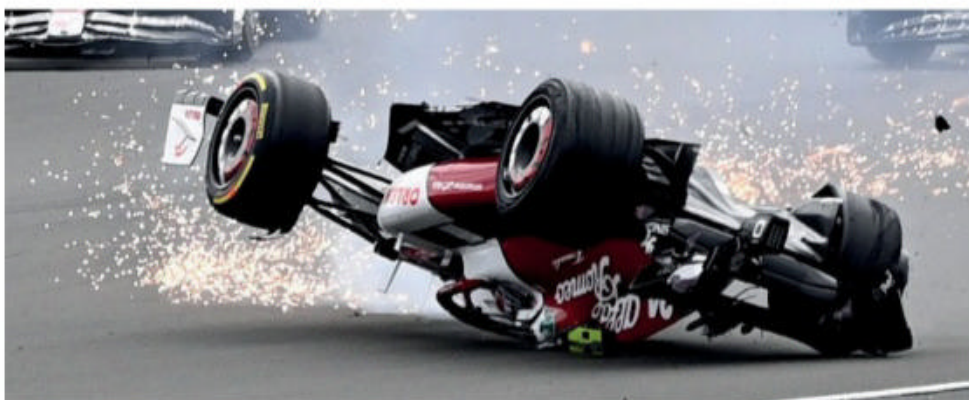
The roll hoop requirements have been beefed up following on from Zhou Guanyu's British GP shunt
