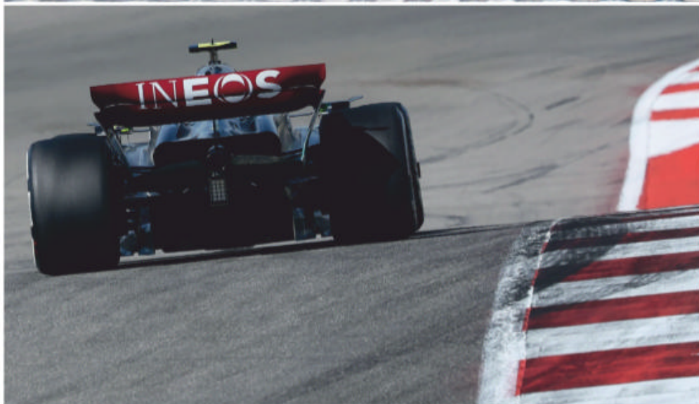
Current aero regulations means teams are aiming to run their cars as low to the ground as possible, some with more success than others
